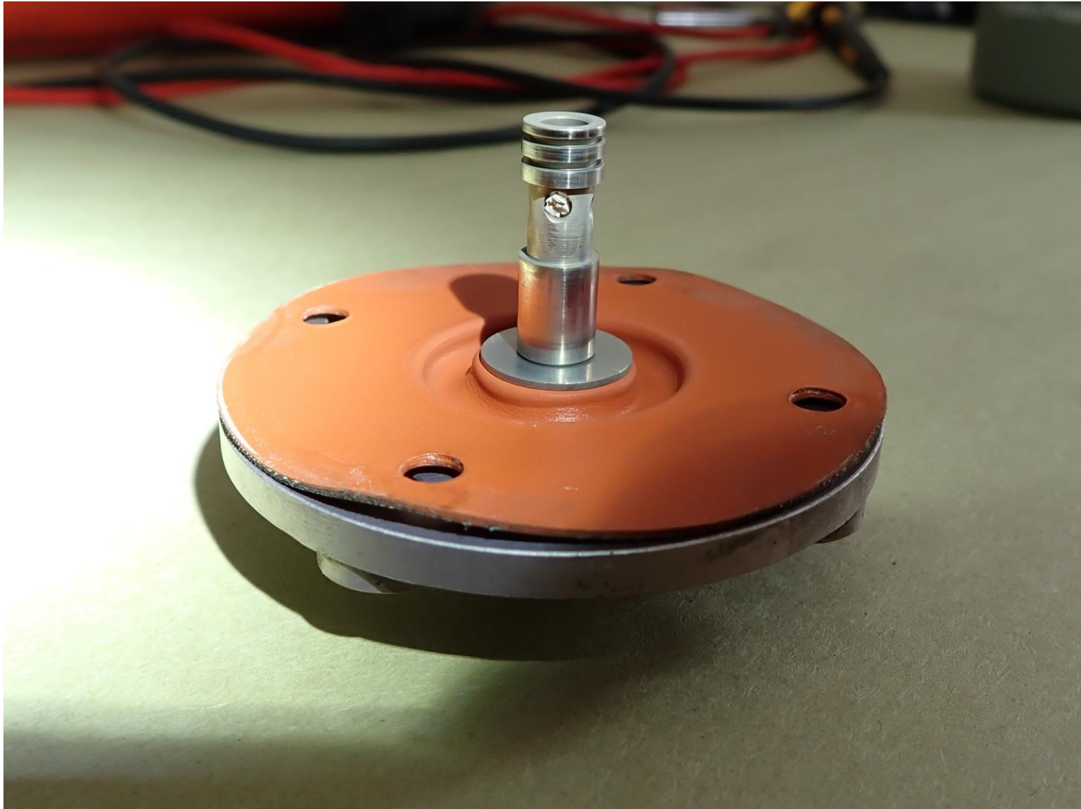
Photograph 5 - Partially Blocked Diaphragm Metering Stem
