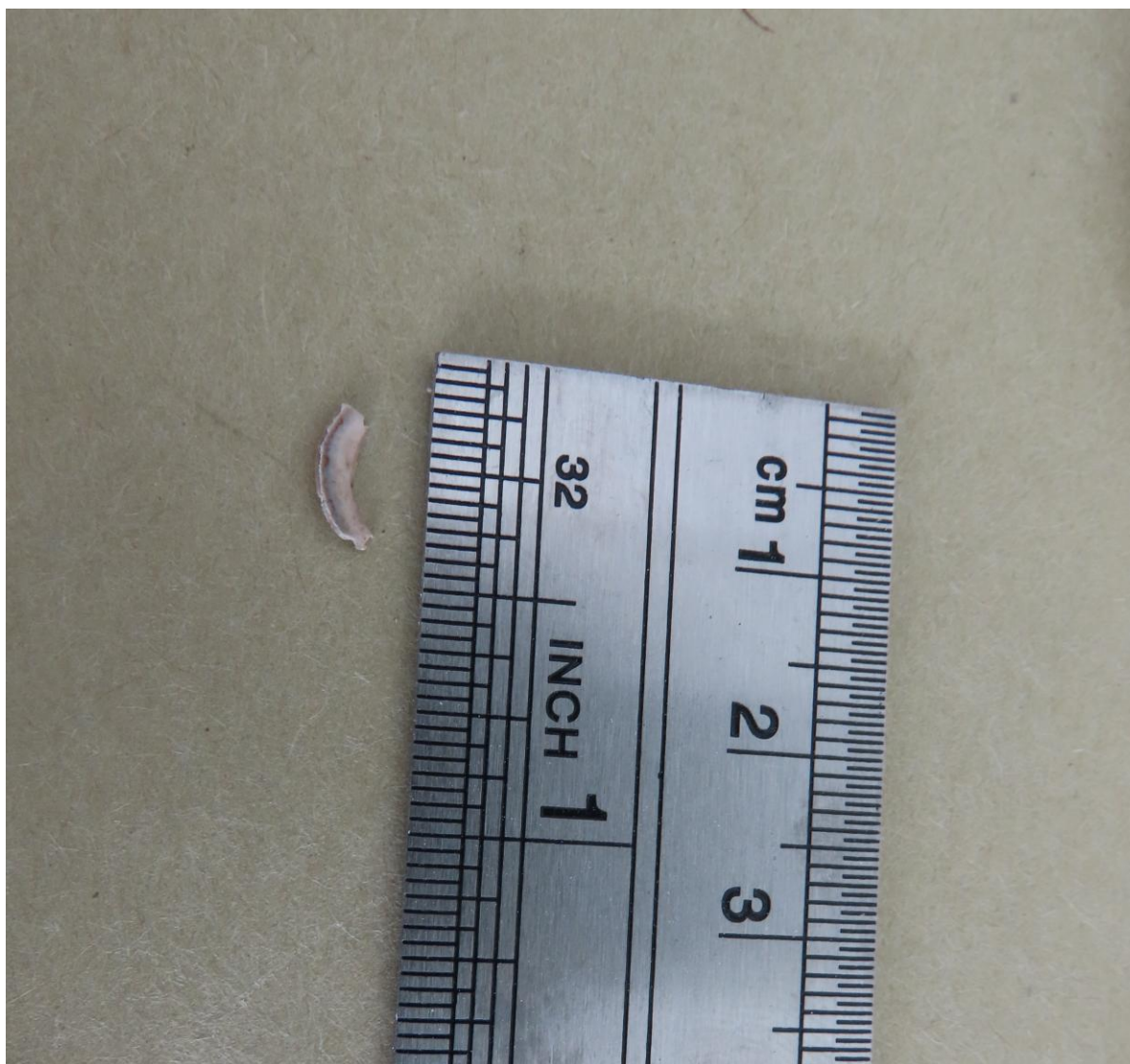
Photograph 7 - Debris From Diaphragm Metering Stem
