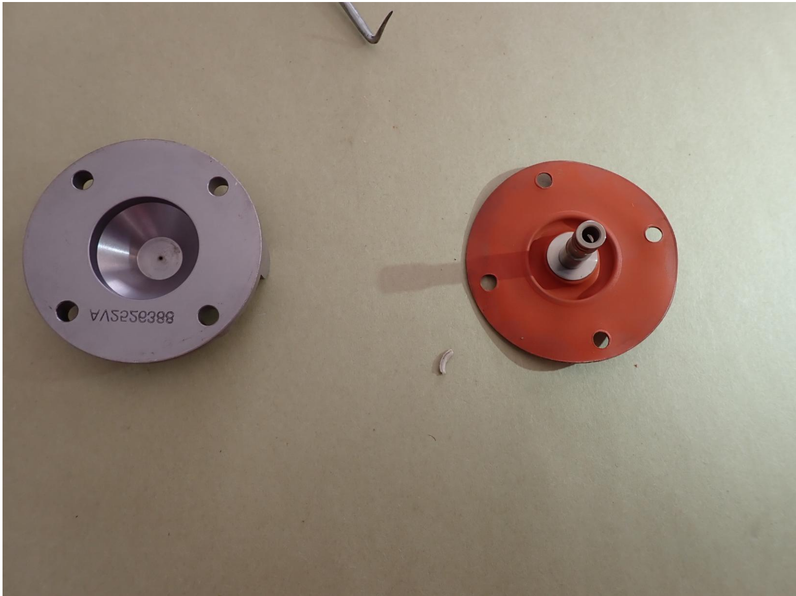
Photograph 6 - Extracted Debris From Diaphragm Metering Stem
