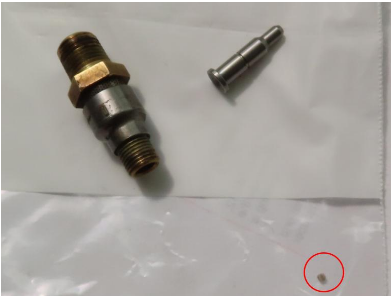
Photograph 4 - Debris Found in Fuel Injector Nozzle/Engine Cylinder No. 1
