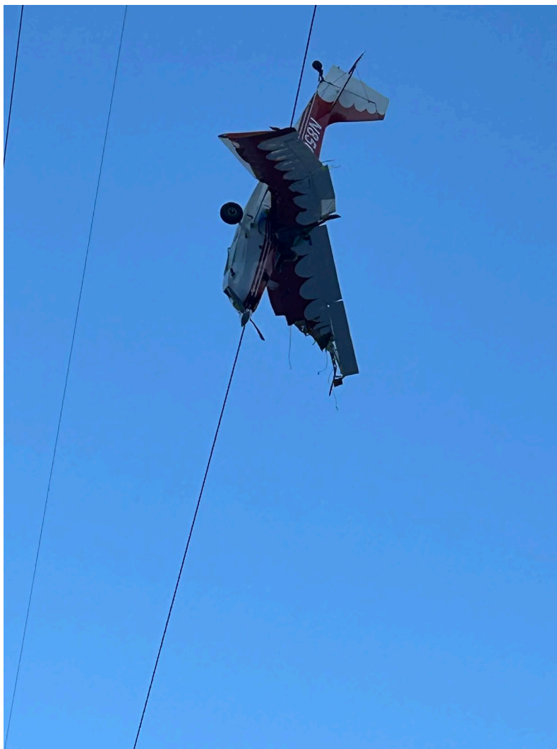
Photograph 2 - Accident airplane entangled In high-tension powerline (Courtesy of FAA).
