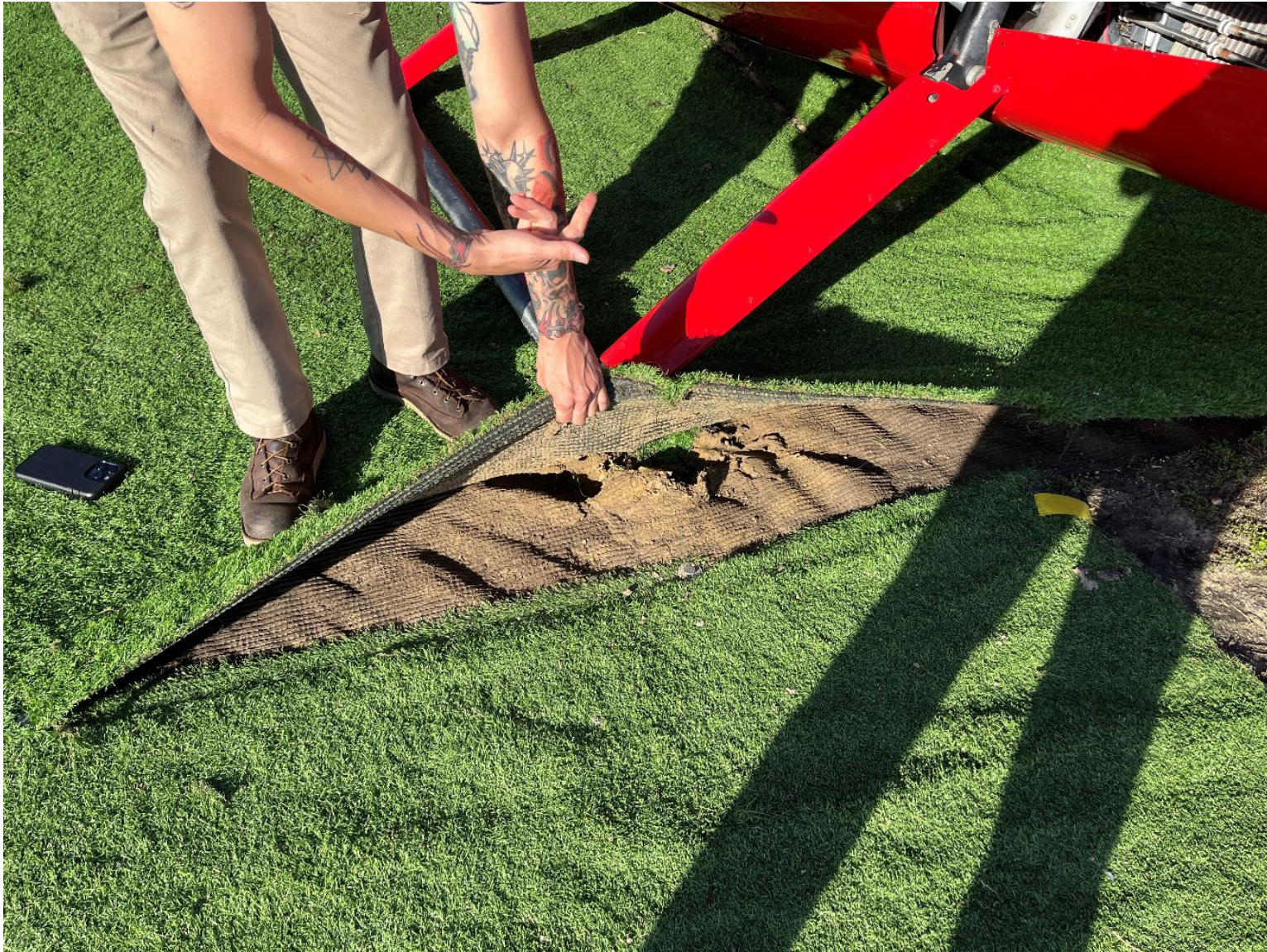
Photograph 6 - View of the helipad material, an artificial turf (courtesy of the Federal Aviation Administration)
