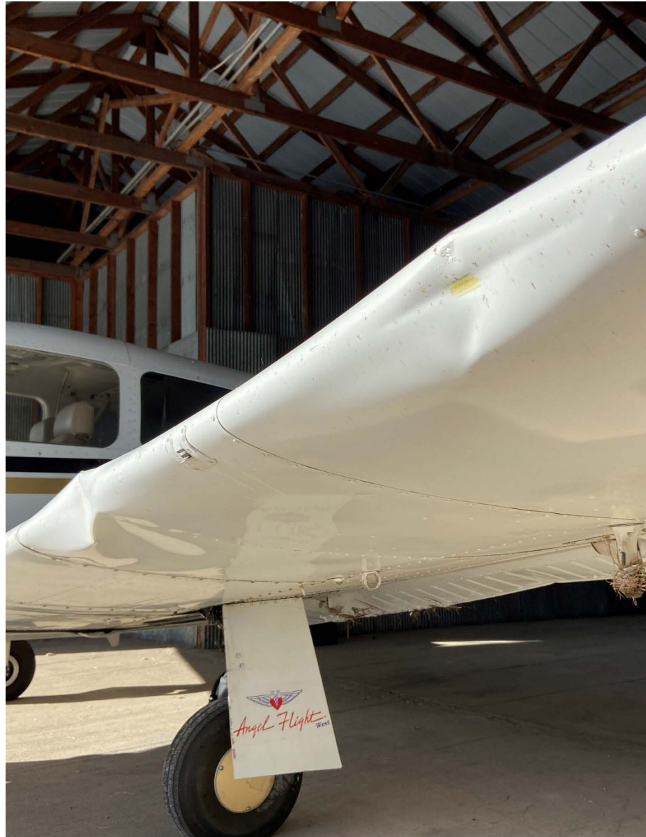
Photograph 2 - Left Wing Substantial Damage (Courtesy of FAA)
