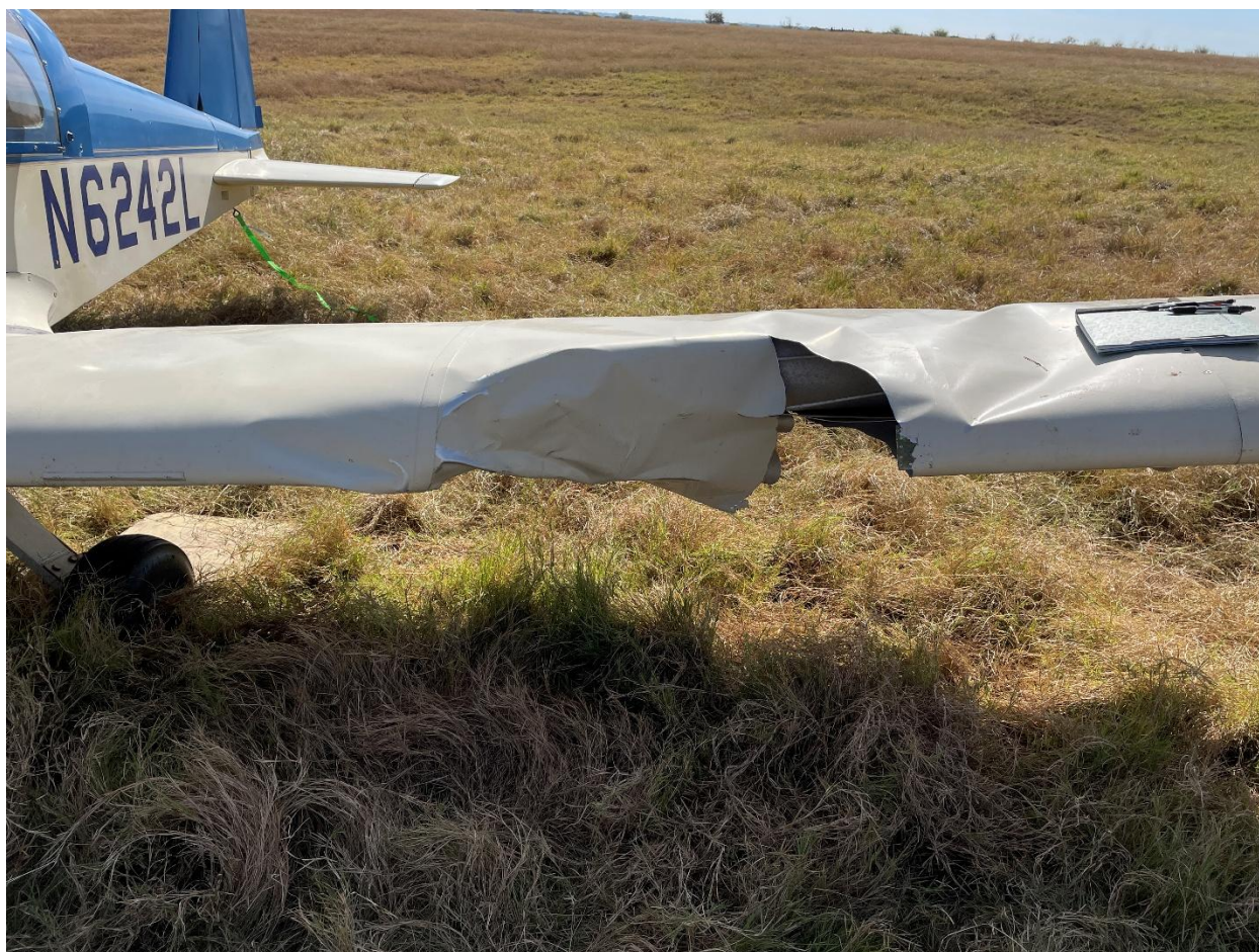
Figure 2. Left wing damage. (Photo courtesy of FAA)
