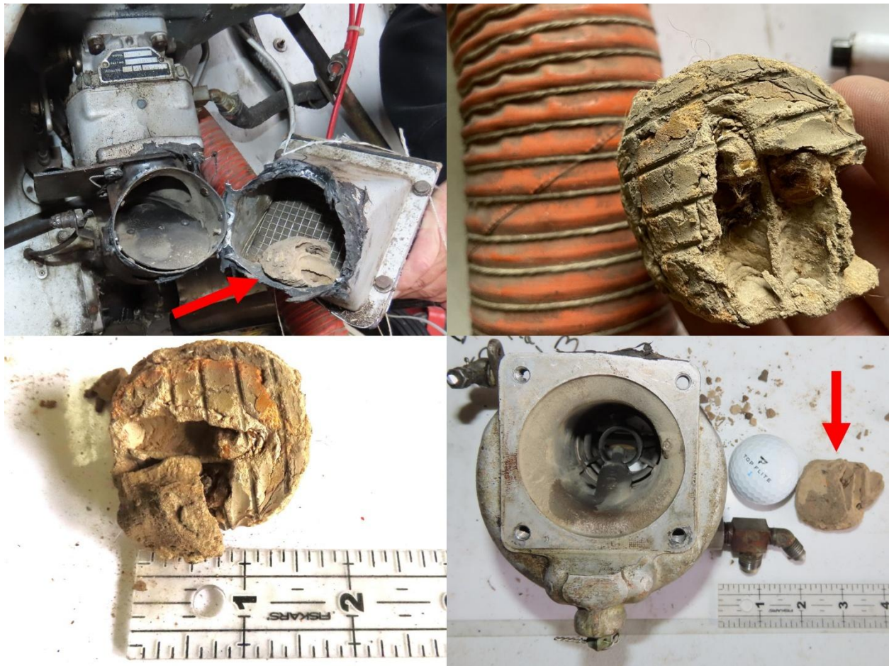
Figure 3. Mud dauber nest found in the airbox between the air filter and the throat of the carburetor. Red arrows point to the mud dauber nest. (Photos courtesy of Lycoming Engines and edited by NTSB)
