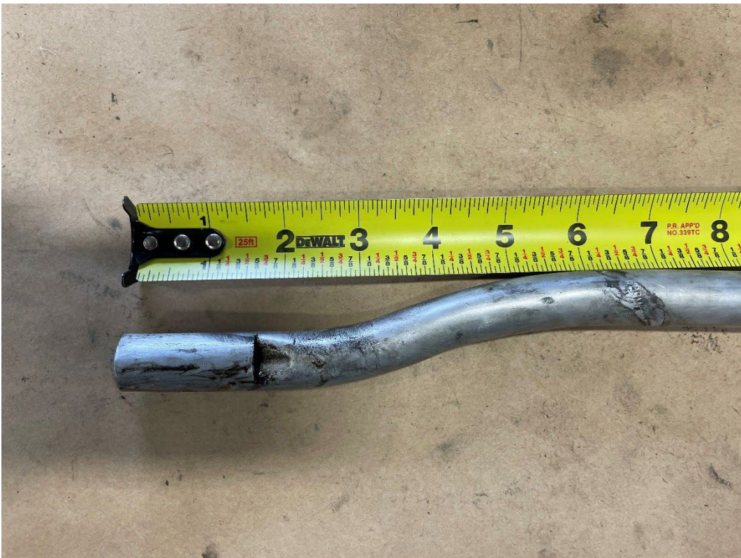
14. Bottom/end of breather tube with secondary hole.
