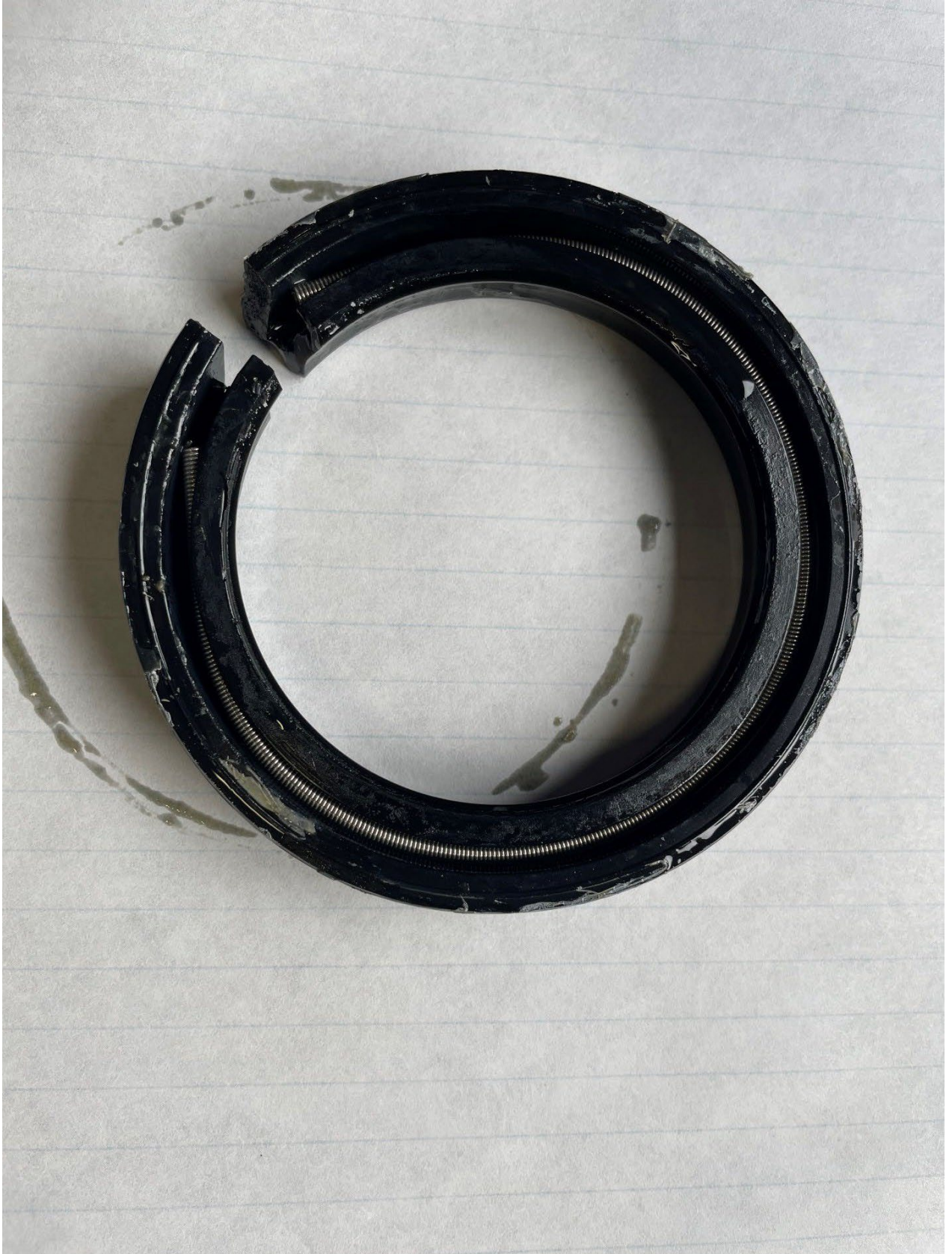
8. Nose seal removed from engine - rear face.
