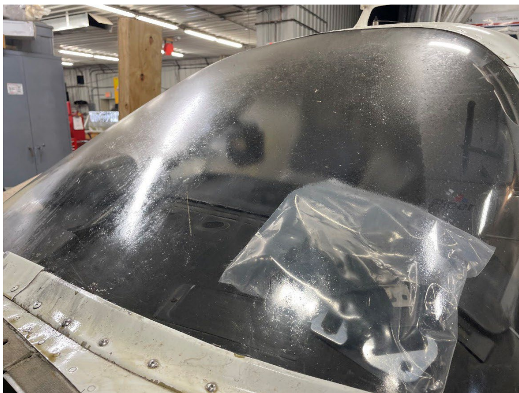
2. Oil residue noted on forward windscreen.
