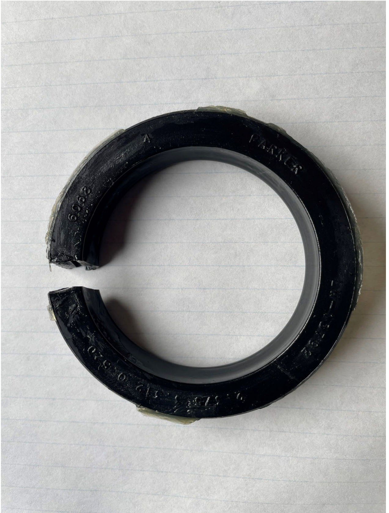
7. Nose seal removed from engine - front face.
