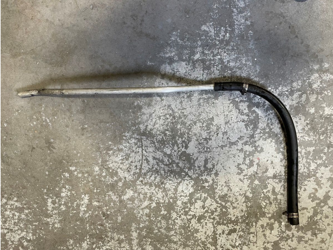
13. Aircraft oil breather tube, as removed.
