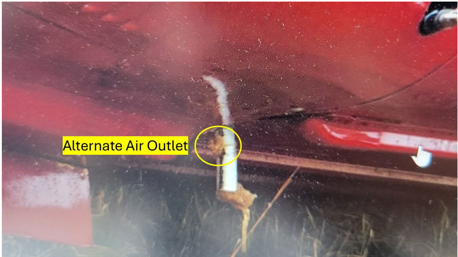
Photograph 2 - Ice obstructed engine oil breather tube and alternate air outlet (Source: Recovery Company)
