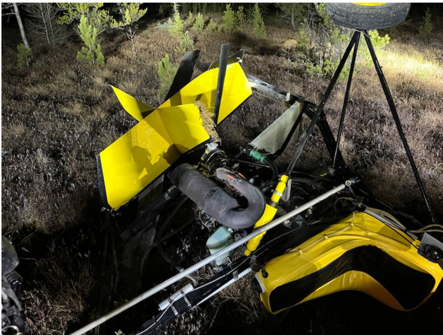
Photograph 2 - View of the empennage and the engine at the accident site (courtesy of the Federal Aviation Administration)
