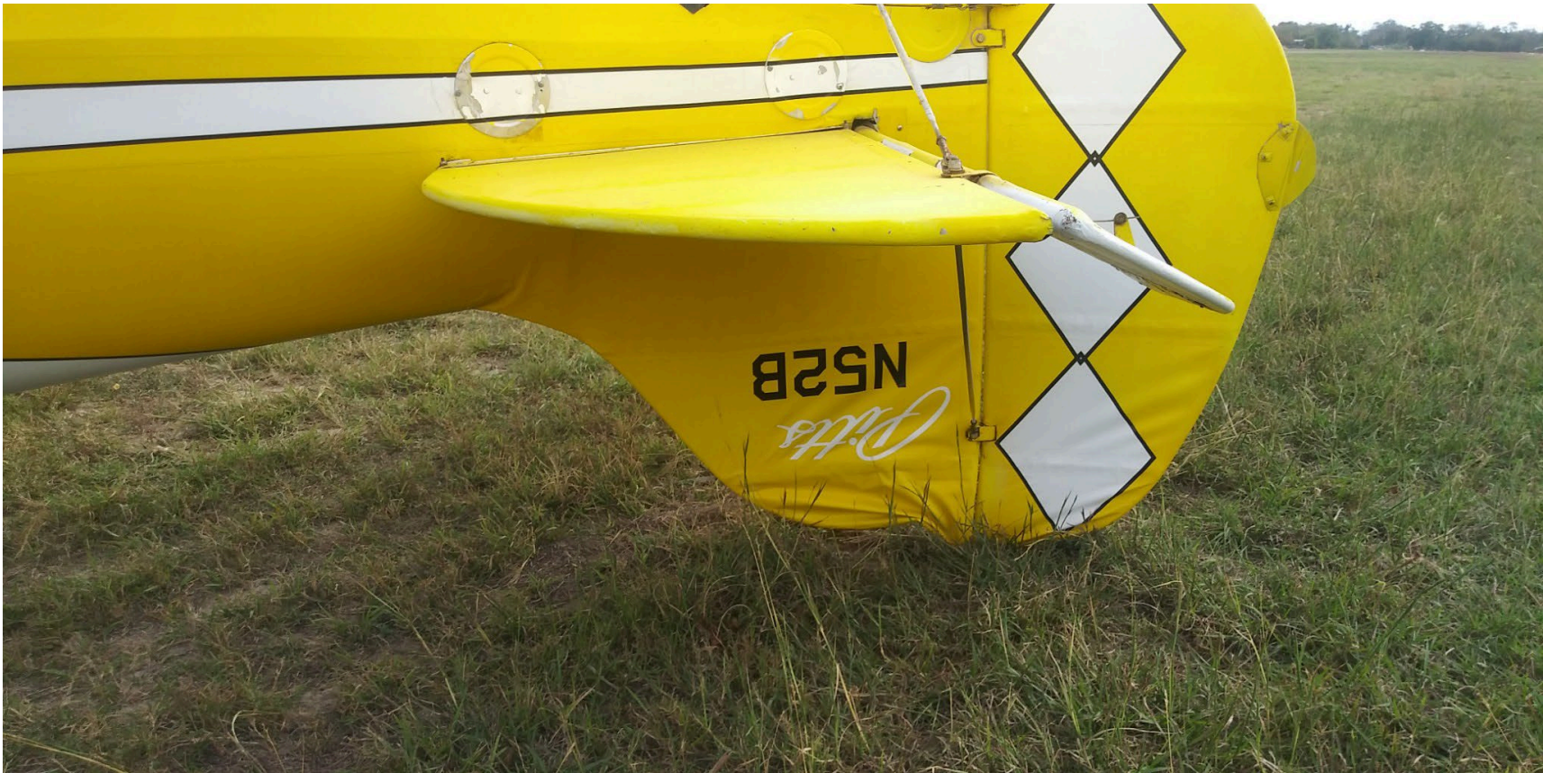
Photograph 2 - Vertical Stabilizer Damage (Courtesy of Federal Aviation Administration)
