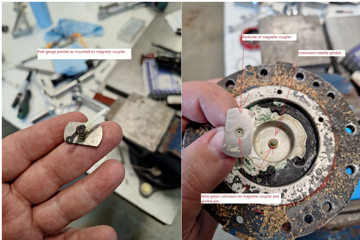
Figure 1 - The left wing fuel gauge pointer (left) and the underside of the fuel gauge (right)
