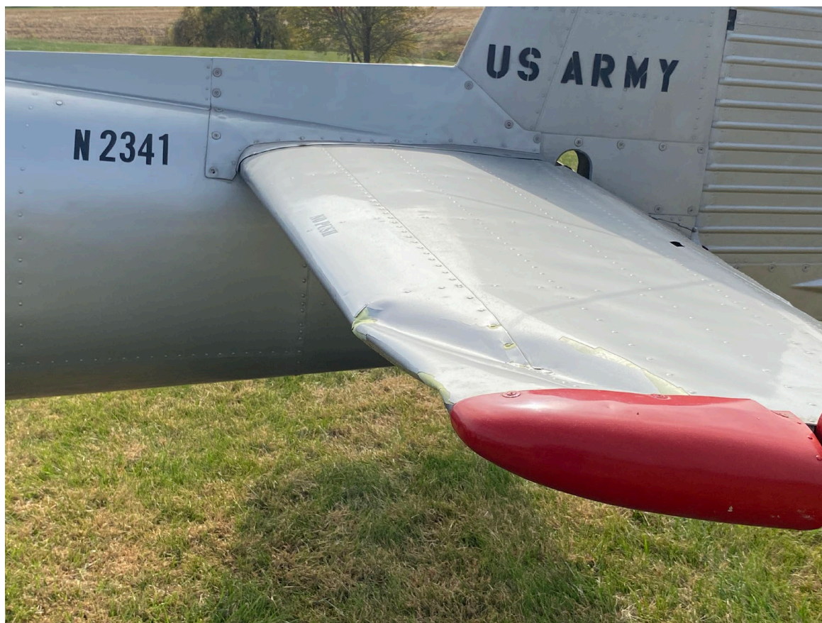
Photograph 2 - Damaged left horizontal stabilizer (Courtesy of FAA)
