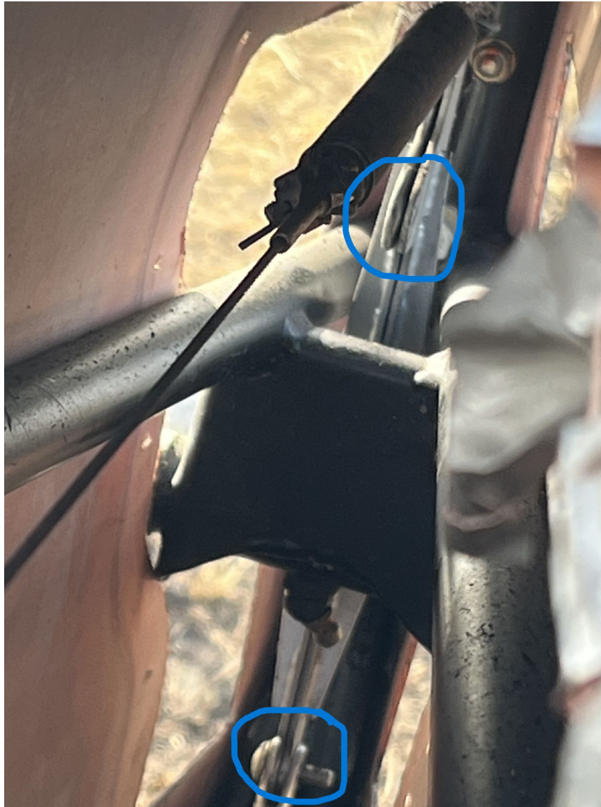
Photograph 2 - Elevator Horn (Courtesy of FAA)
