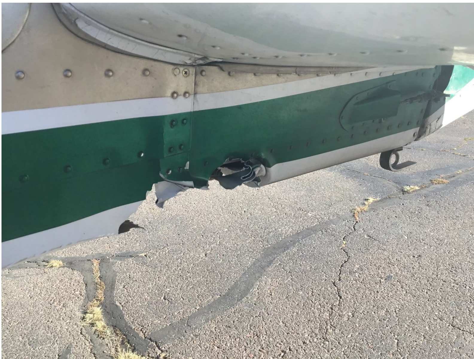
Photograph 2 - Fuselage Substantial Damage (Courtesy of FAA)
