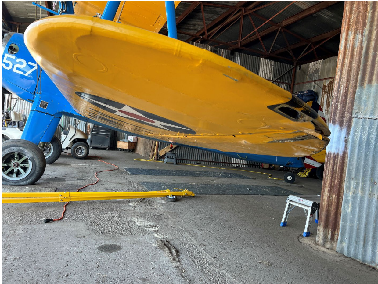
Photograph 2 - Left lower wing damage (Courtesy of FAA)
