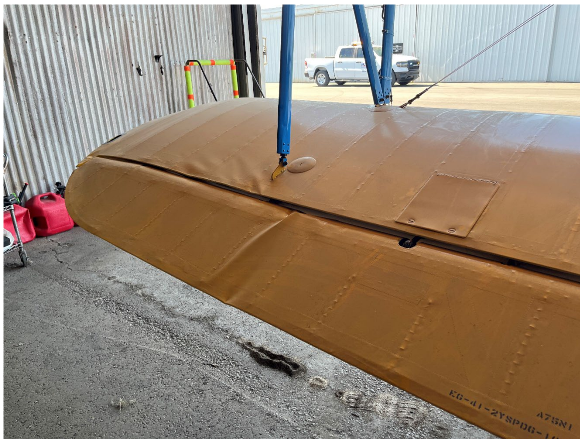
Photograph 3 - Left lower wing aileron damage (Courtesy of FAA)
