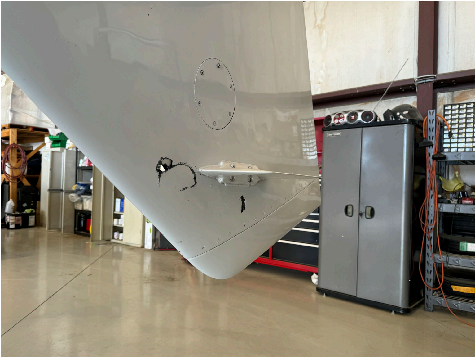
Photograph 2 - Ventral Stabilizer Damage (Courtesy of Addison Airport Manager)
