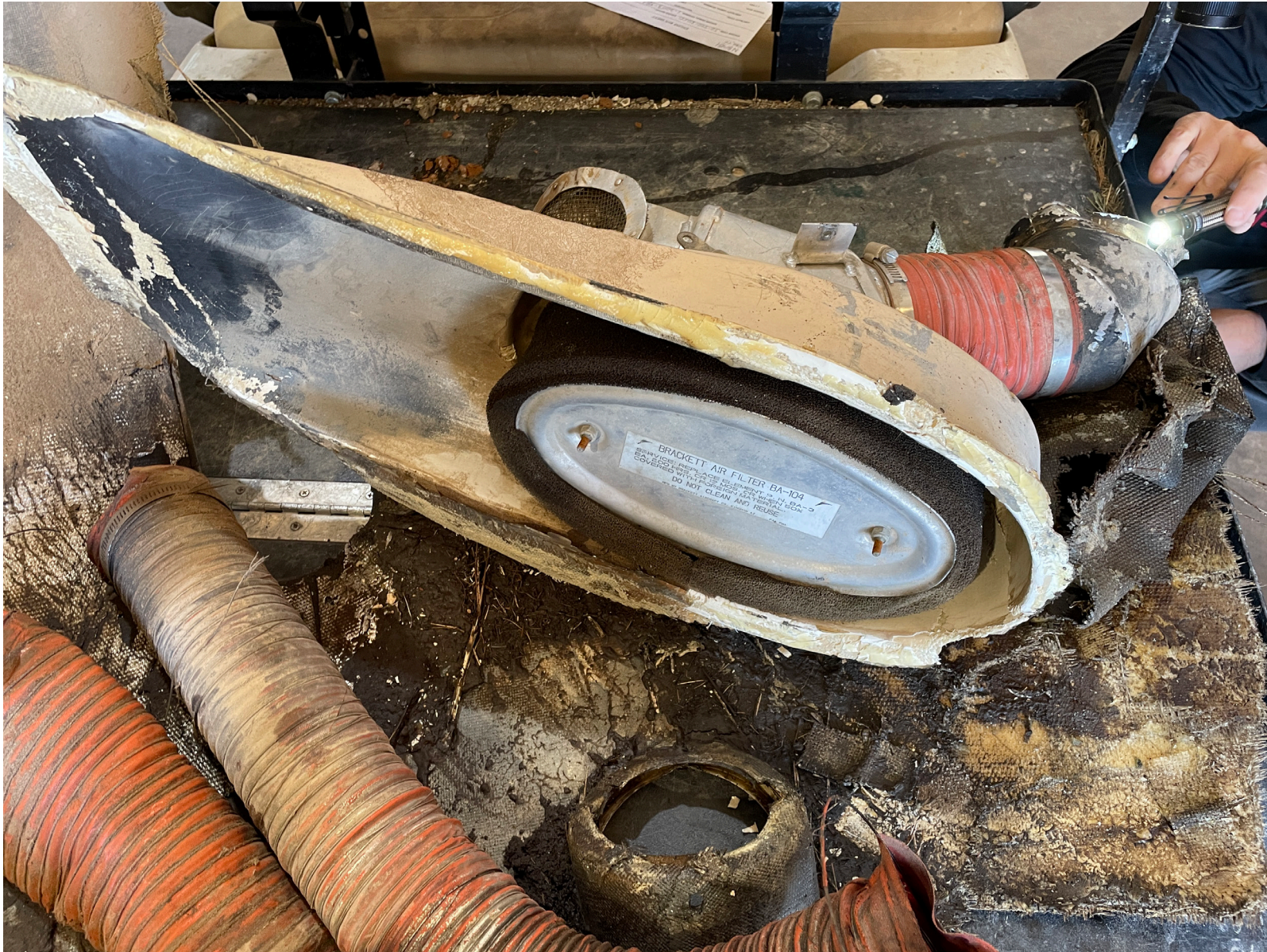
Photograph 6 - Air filter, air box, scat duct (Courtesy of NTSB)
