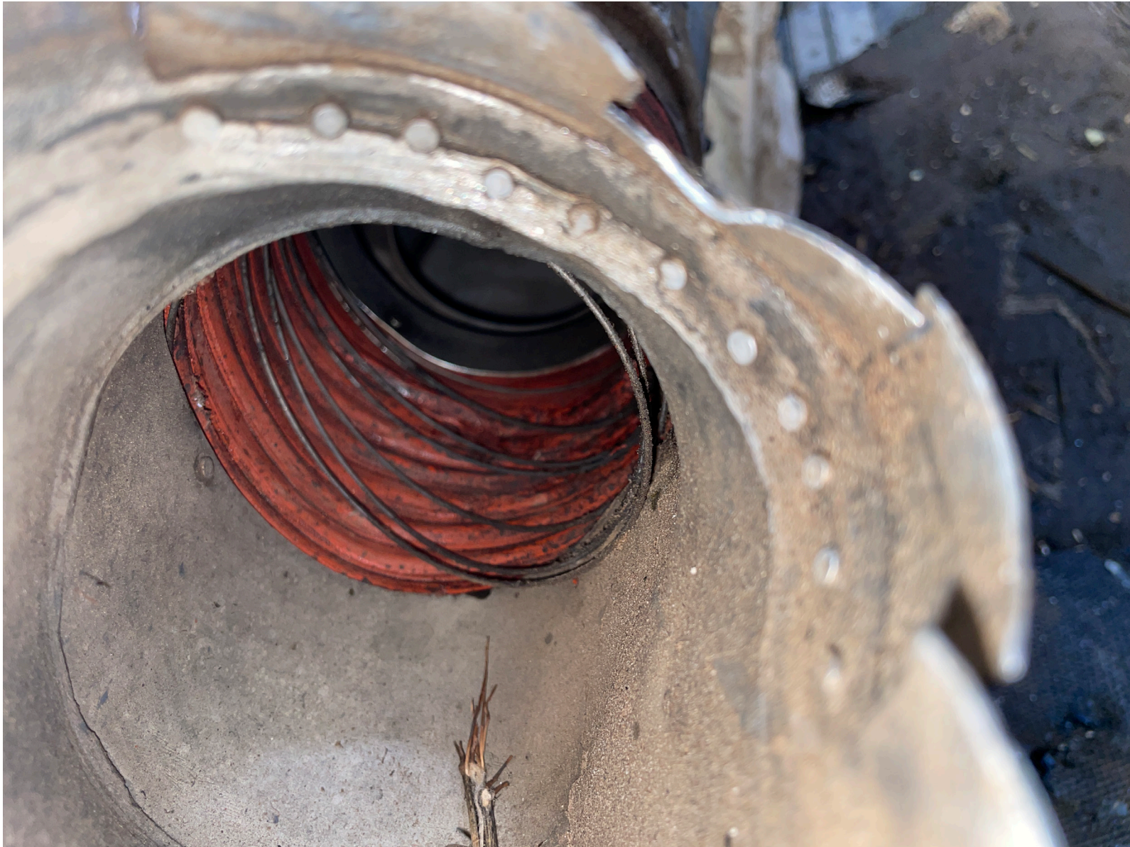
Photograph 7 - Collapsed and degraded scat duct (Courtesy of NTSB)
