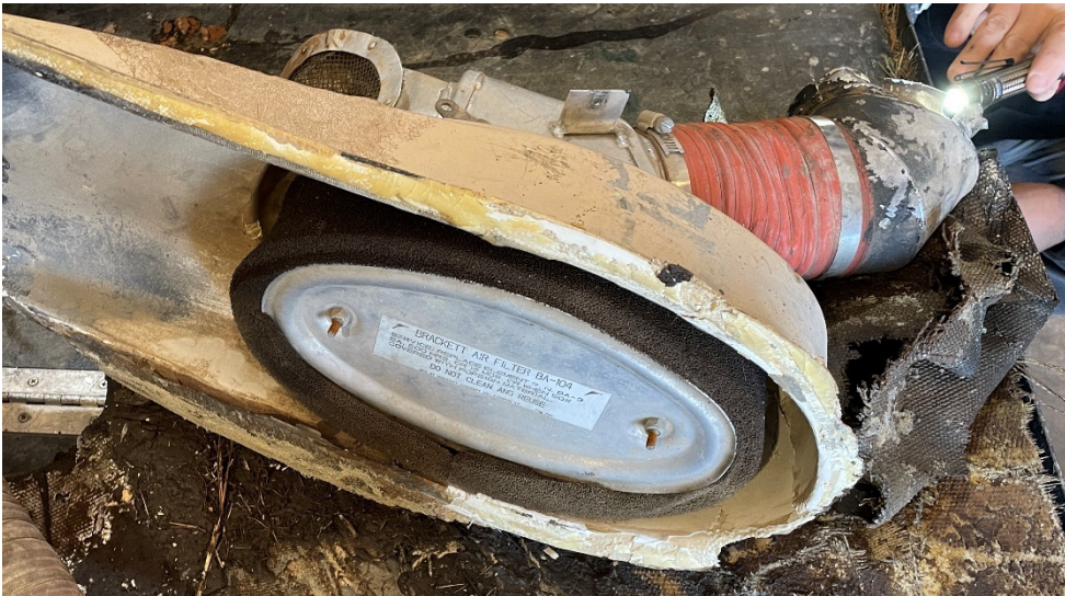
Figure 3. Air scoop, air filter, airbox, and failed scot duct at the postaccident exam.
