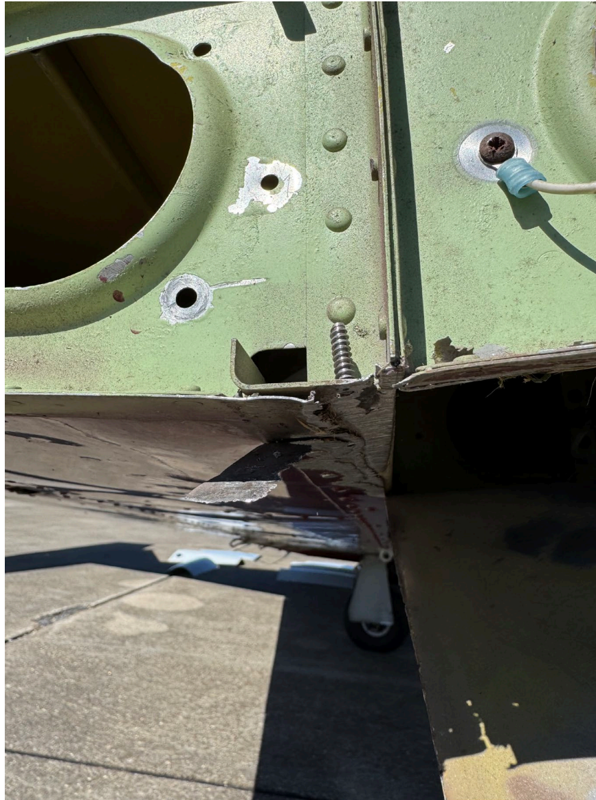
Photograph 3 – Spar damage (Courtesy of accident pilot)
