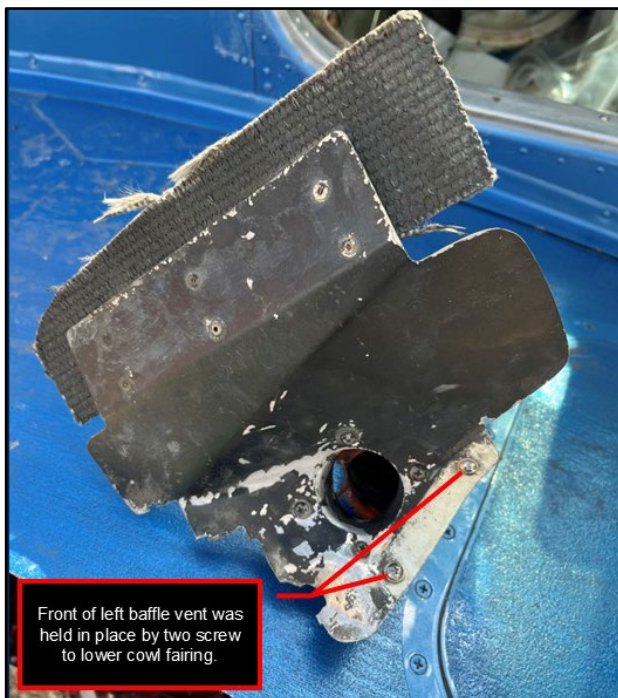
Figure 7. Left Vented Baffle top view after removal from airplane.
