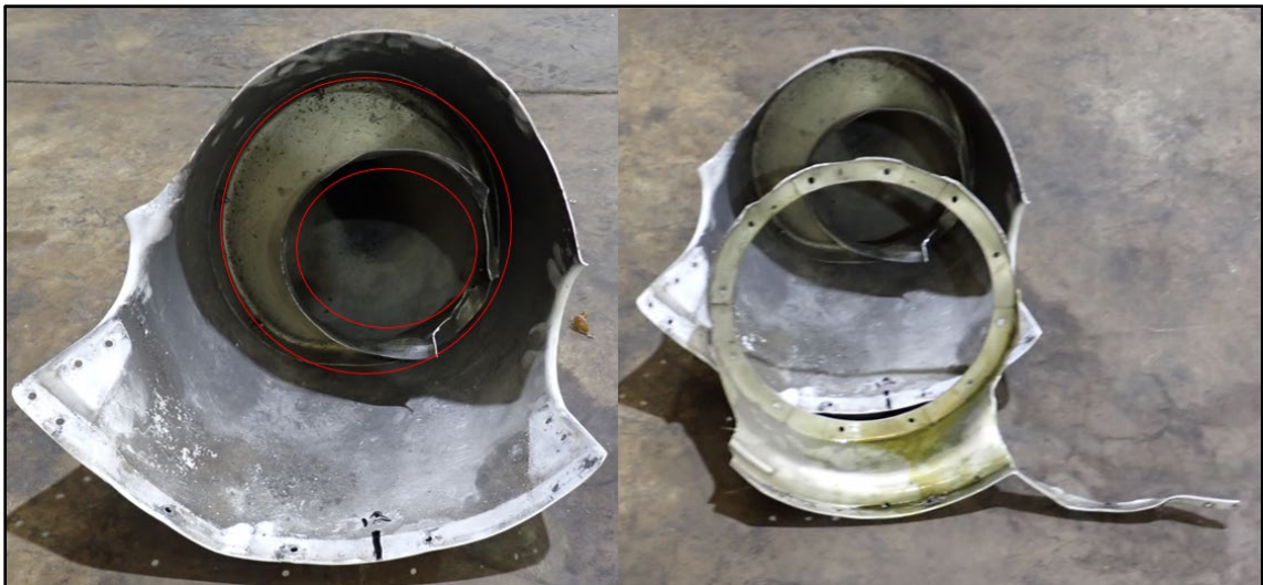
Figure 12. Left photo diagram shows rotational damage to interior bulkhead of the spinner. Photo on right shows the remaining portions of the spinner and spinner bulkhead. 1
