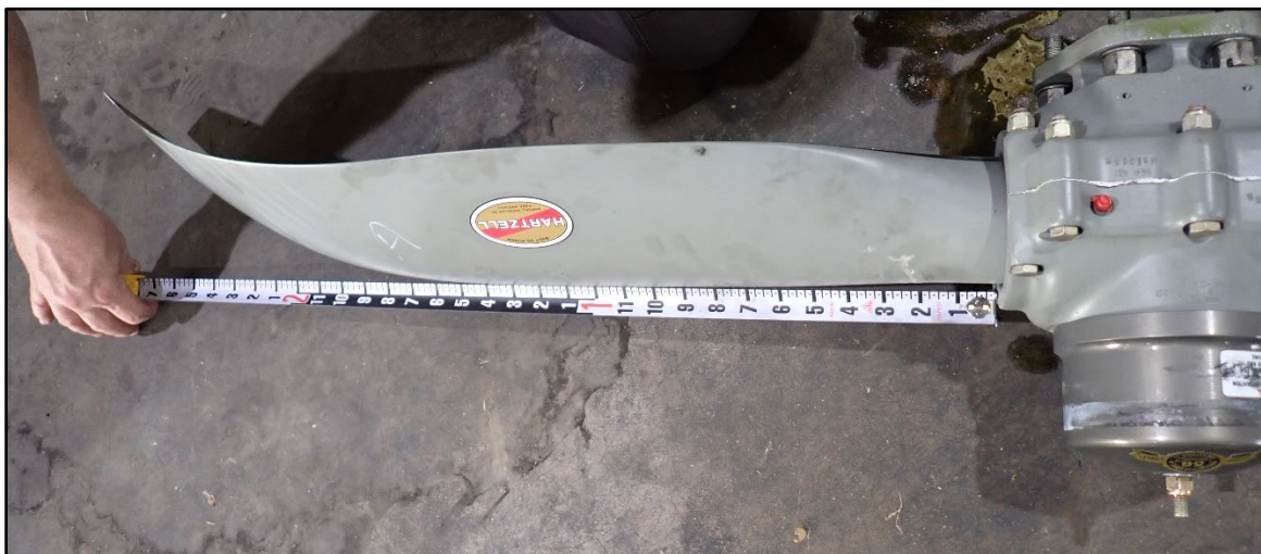
Figure 17. Blade A bent aft near outboard end of blade.
