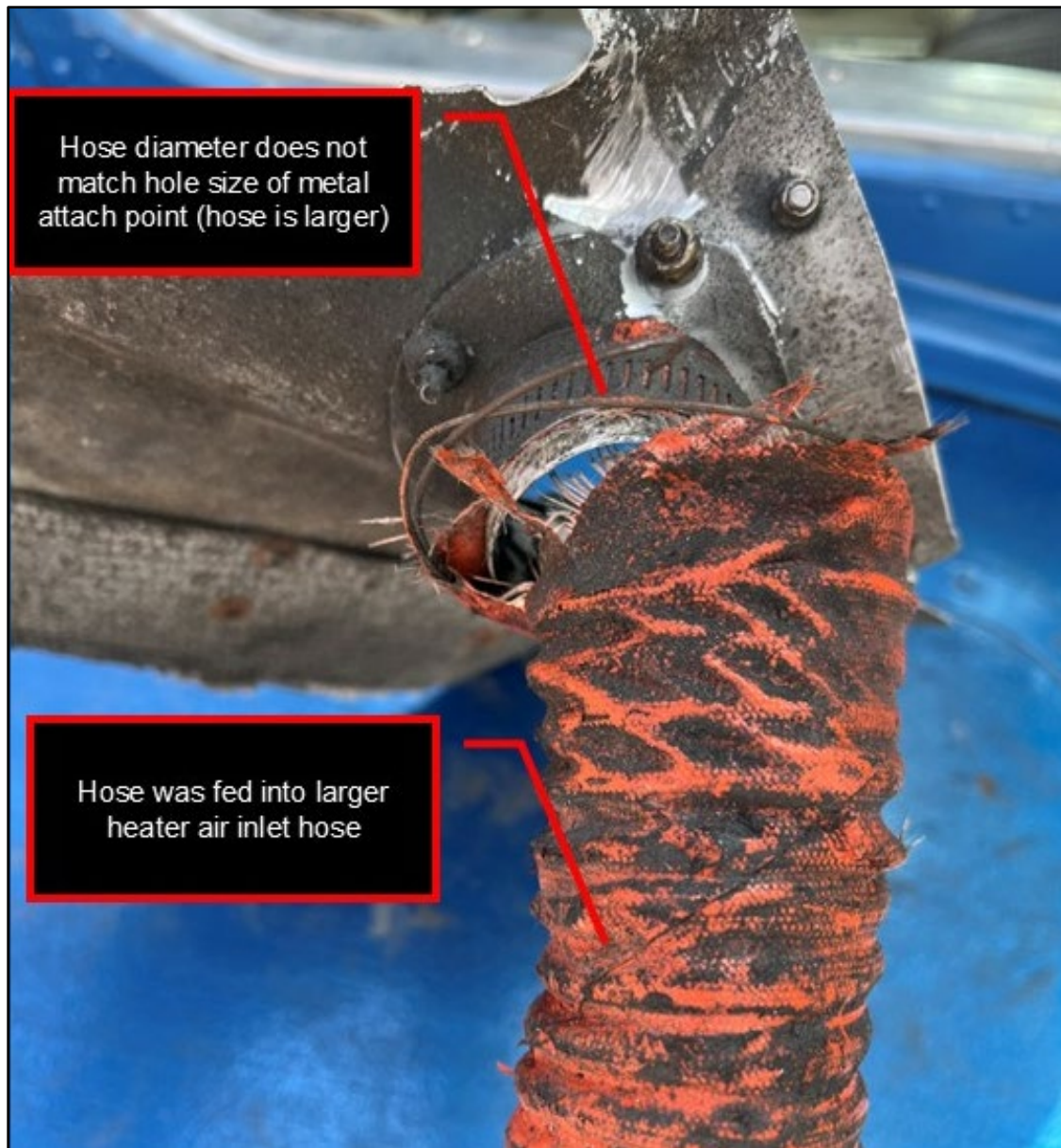
Figure 8. Left Vented Baffle bottom view after removal from airplane.
