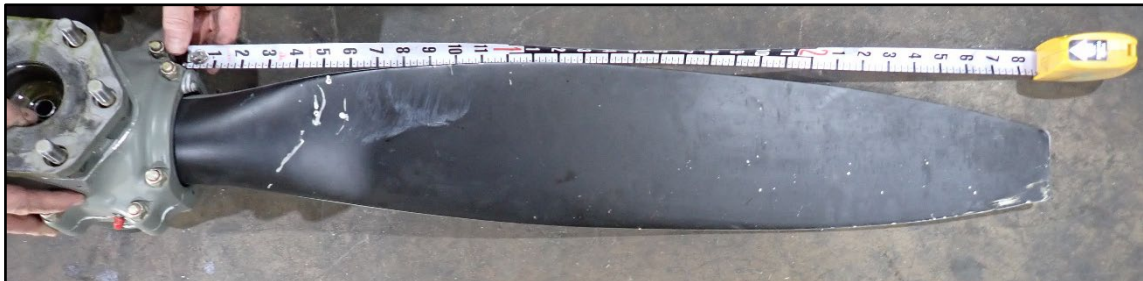
Figure 19. Blade B - blade face. Blade is bent aft at mid-span.
