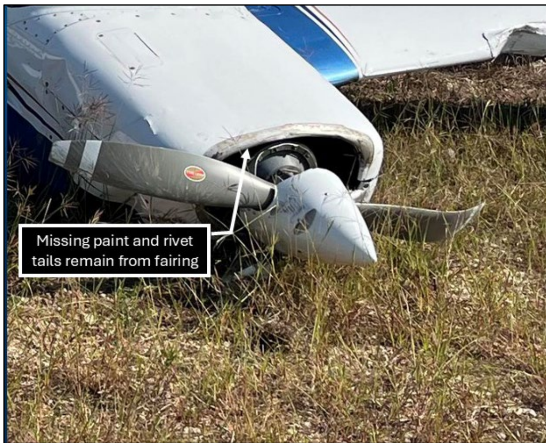
Figure 4. Missing upper cowl fairing (courtesy of FAA).
