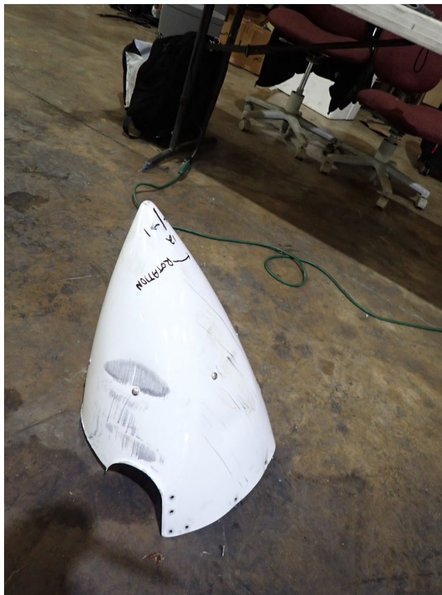
Photograph 8 - Spinner exterior; paint transfer mark
