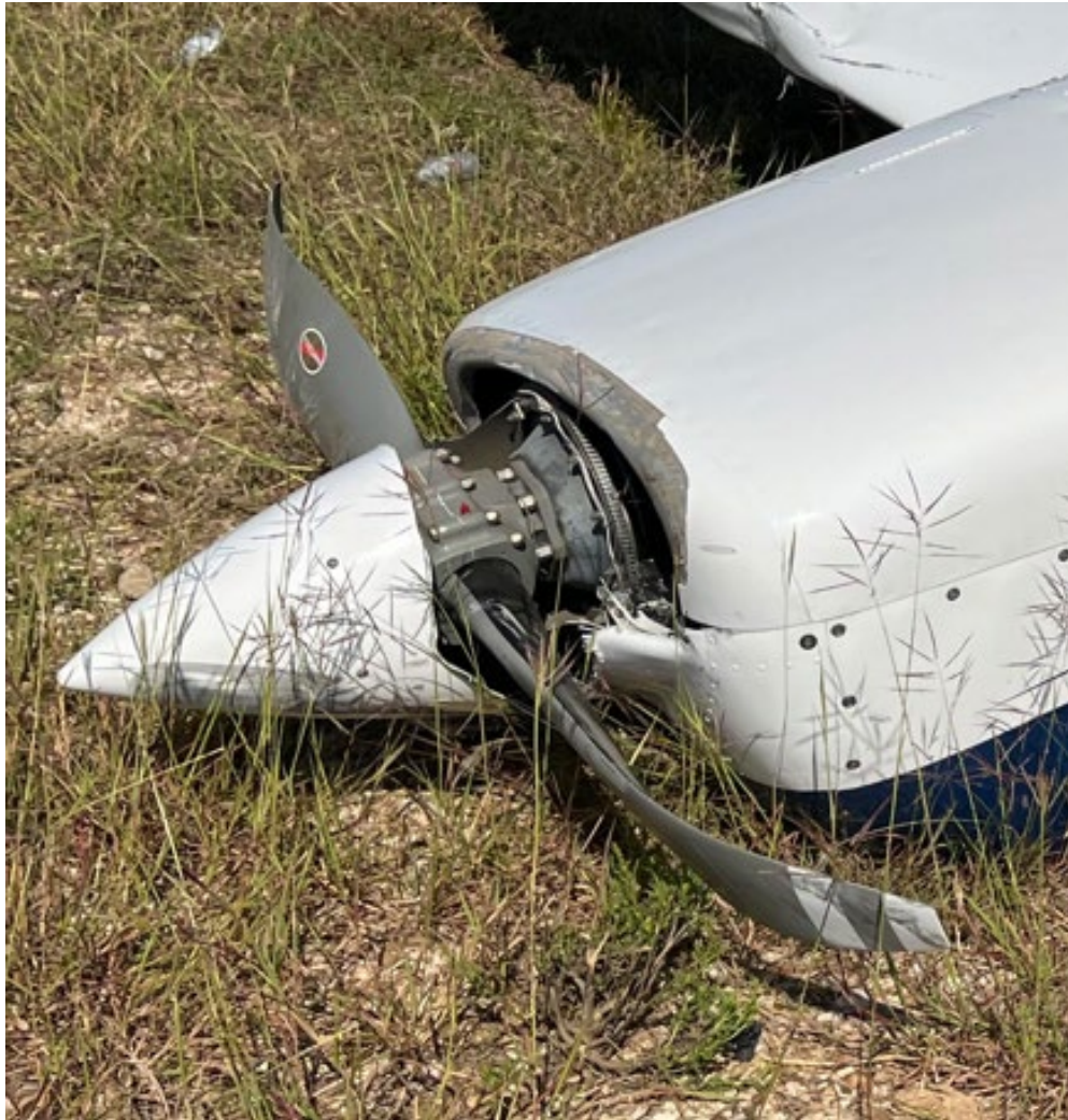
Photograph 5 - Accident site photo Upper & lower cowl fairing damage; spinner & spinner mounting bulkhead damage (courtesy of FAA)
