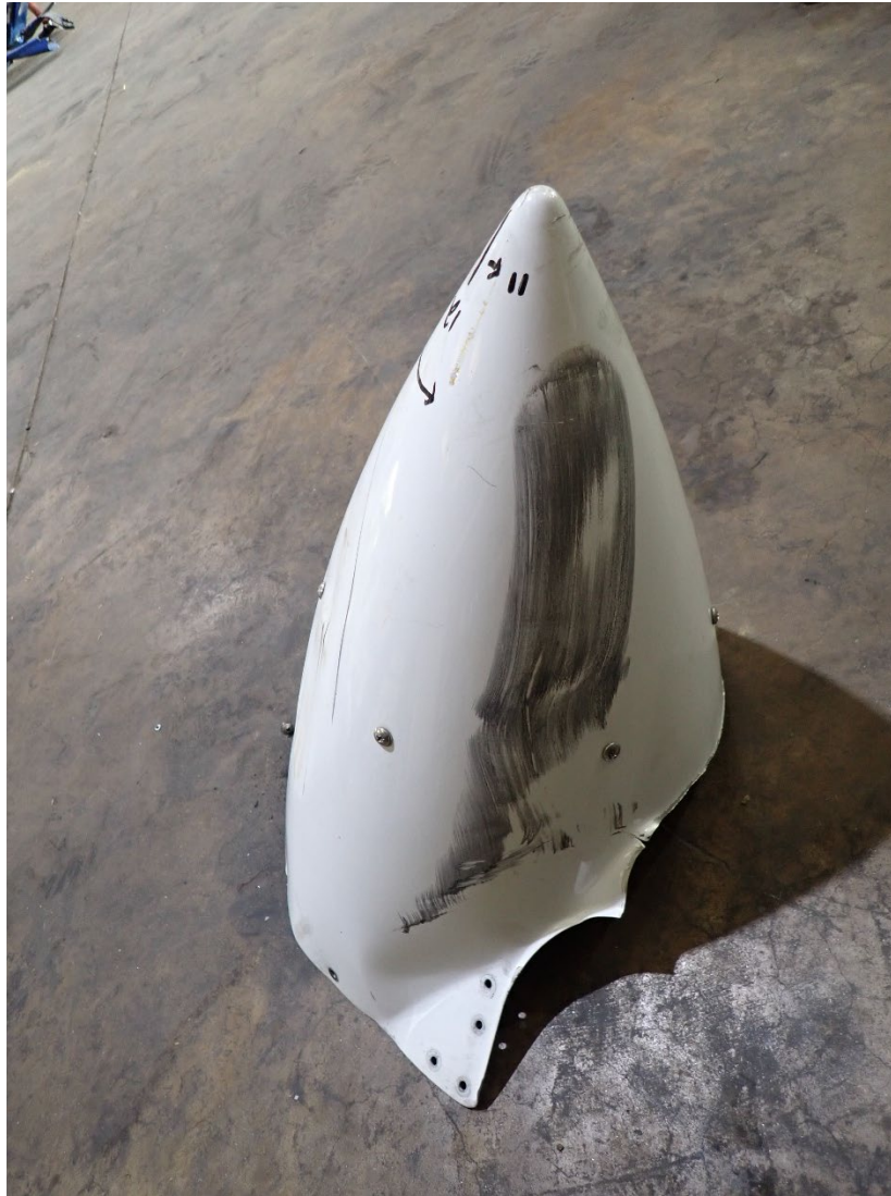
Photograph 7 - Spinner exterior; paint transfer mark
