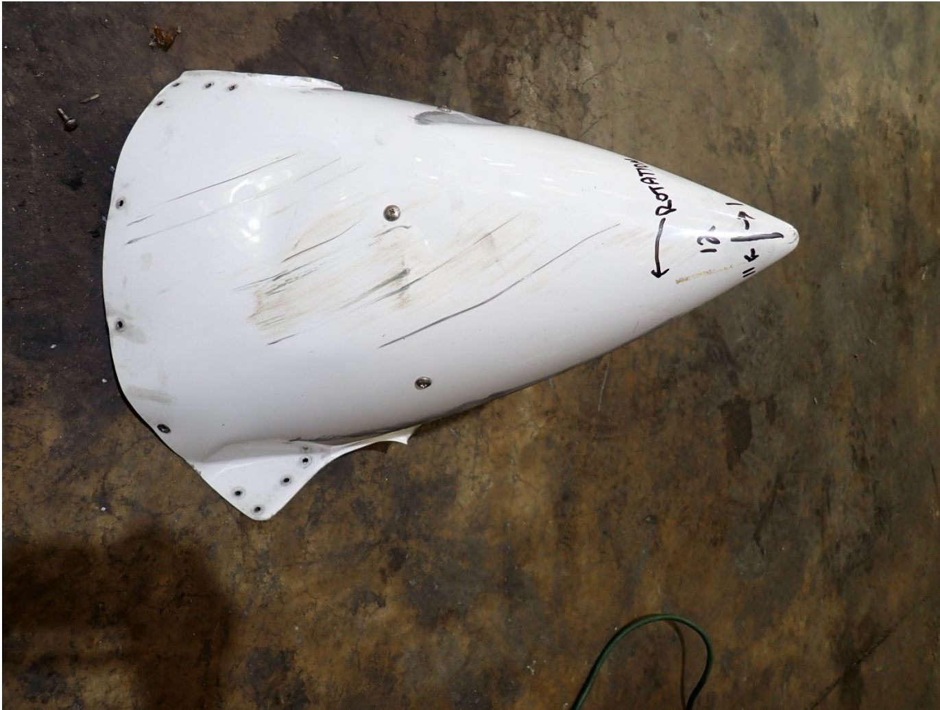
Photograph 9 - Spinner exterior; scratches
