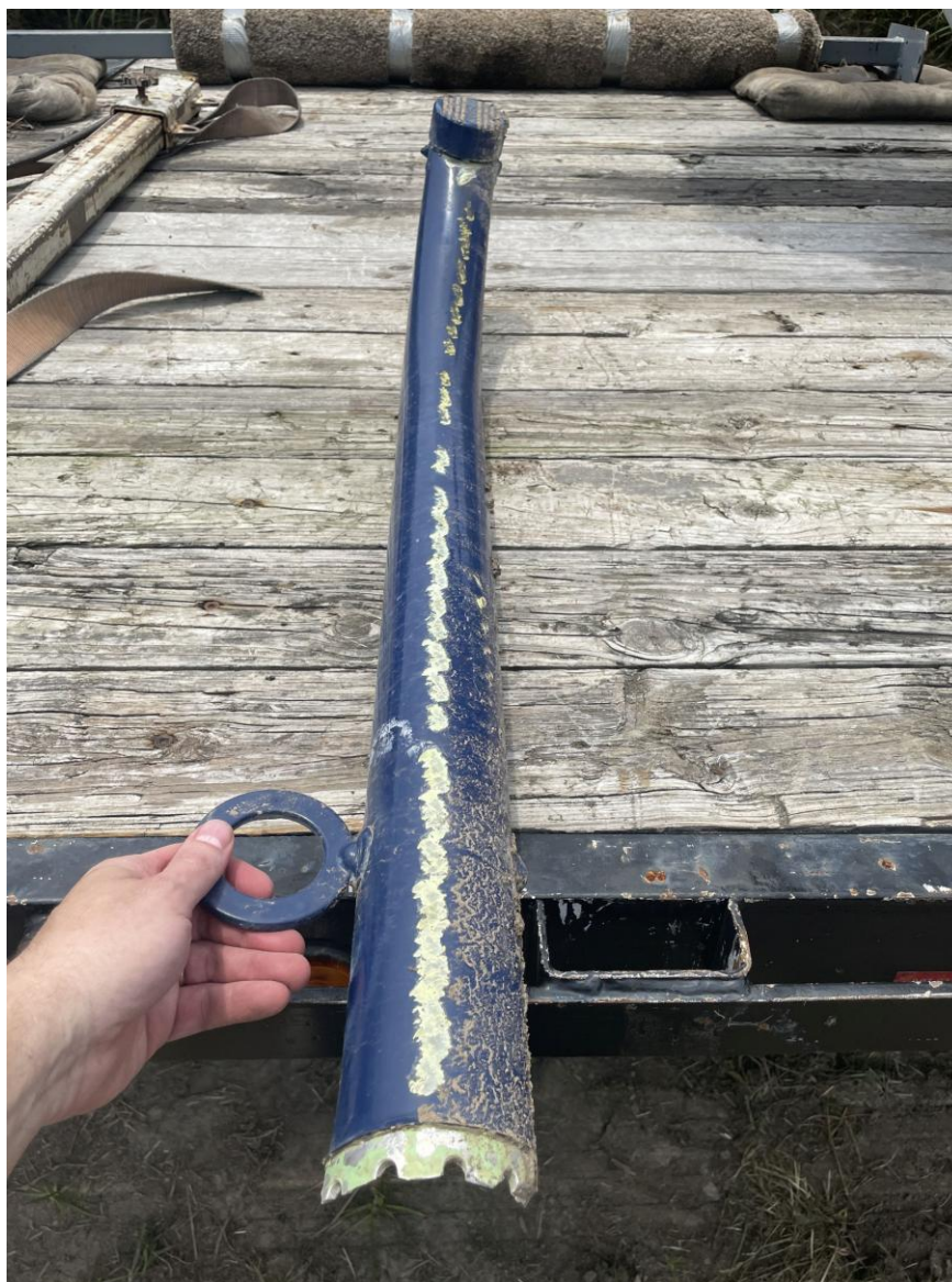
Photograph 7 - Forward landing skid (NTSB photo)
