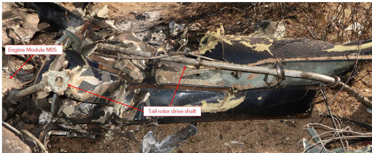
Figure 10. Tail boom inboard section with tail rotor drive shaft attached.
