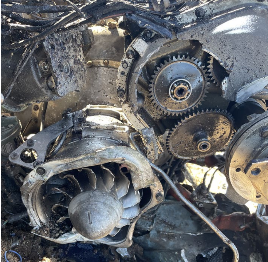
Figure 14. Engine axial compressor (module M02) exhibiting leading edge gouging and blade bending opposite the direction of rotation (Source: Safran Helicopter Engines)
