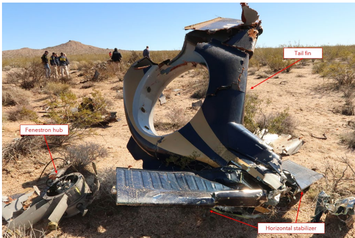
Figure 11. Outboard section of tail boom, horizontal stabilizer, tail fin, and fenestron.
