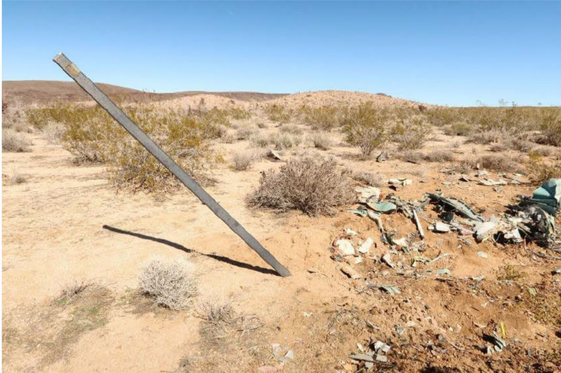
Figure 7. Right side skid step imbedded into the ground at the initial impact area.
