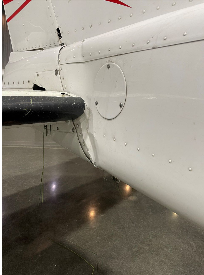
Photograph 2 - Damaged Empennage (Source: Current Airplane Owner).
