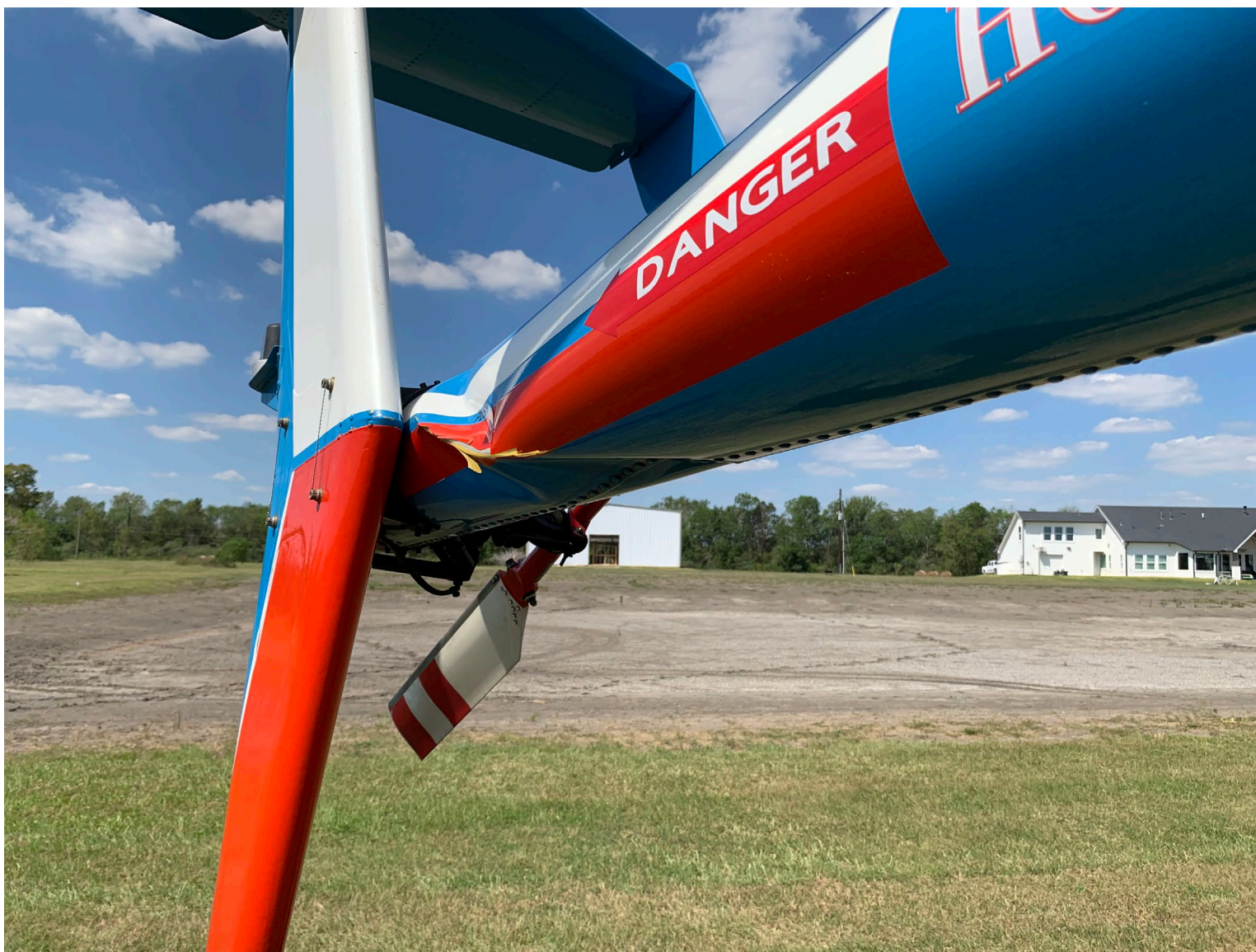
Photograph 1 - Tail Boom Damage (Courtesy of Federal Aviation Administration)
