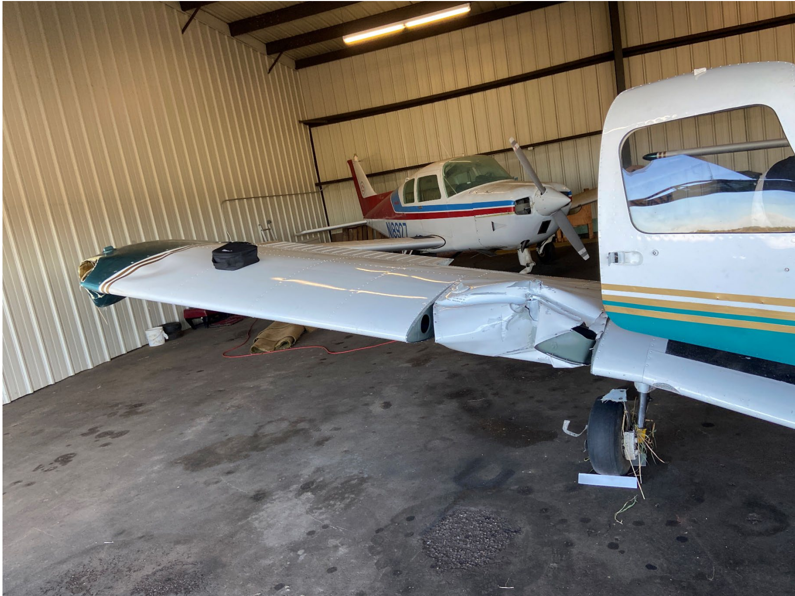
Photograph 2 - Right Wing Damage (Courtesy of FAA)
