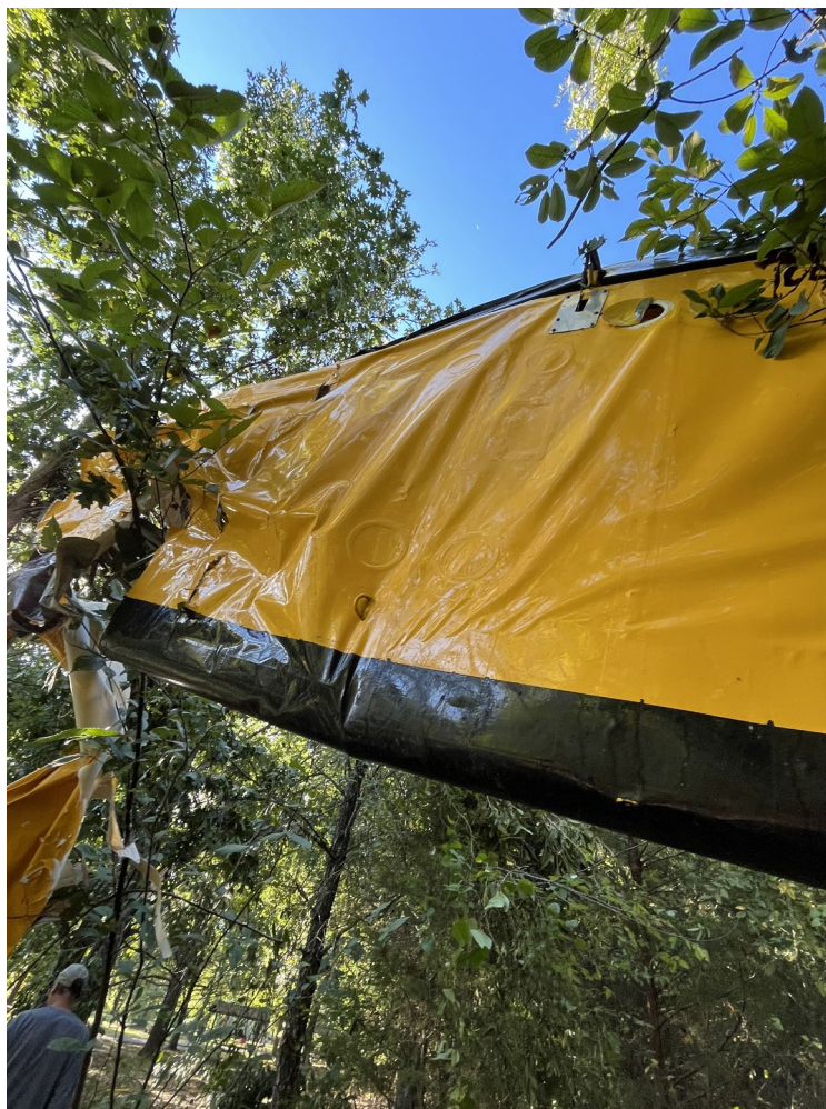
Photograph 2 - Left wind damage (Courtesy of FAA)
