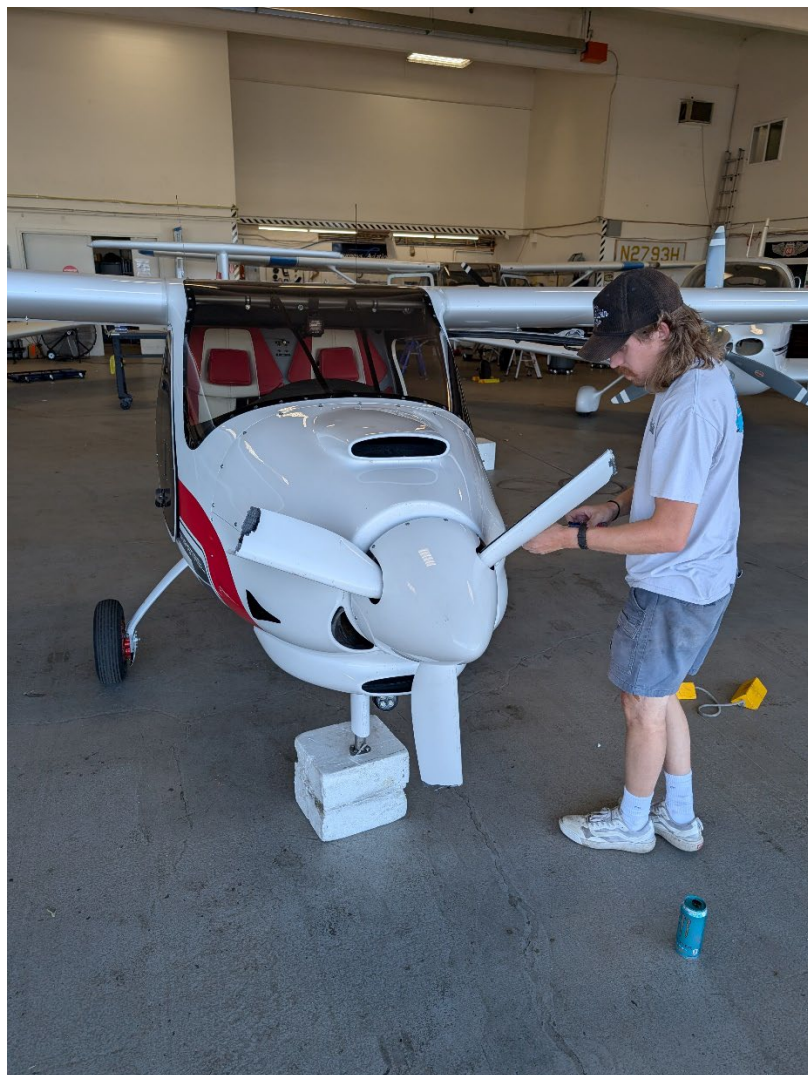
Photograph 1 - Accident airplane propeller and nose landing gear damage (Courtesy of FAA)
