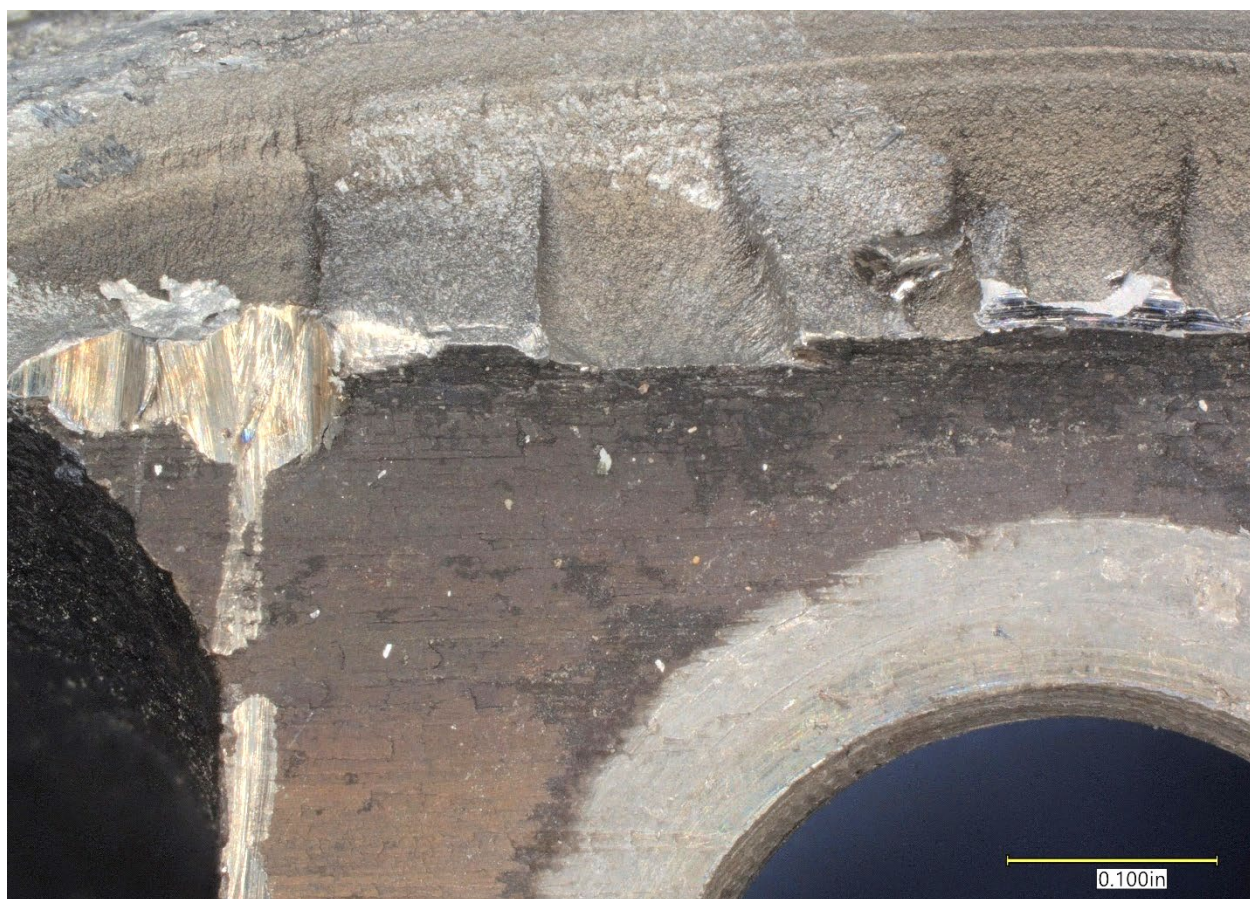
Figure 5. Closer view of several of the initiation sites from the left of Figure 4, separated by vertical ratchet marks.
