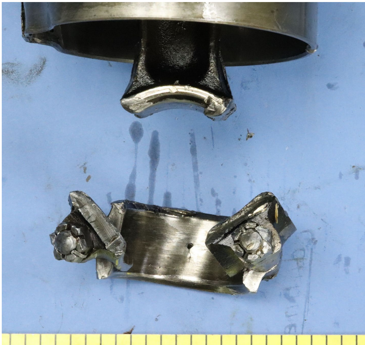
Figure 2. Opposite sides of the fractured connecting rod.
