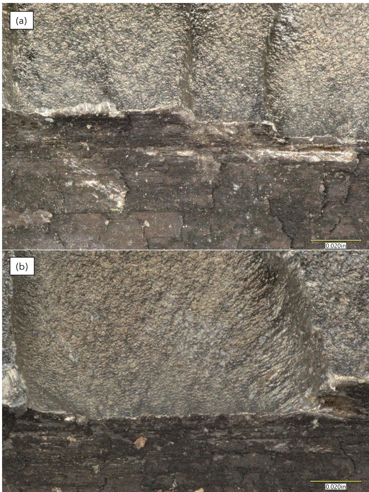
Figure 6. Closer views of (a) several of the crack initiation sites from Figure 5, and (b) a closer view of the central initiation site in 6a.
