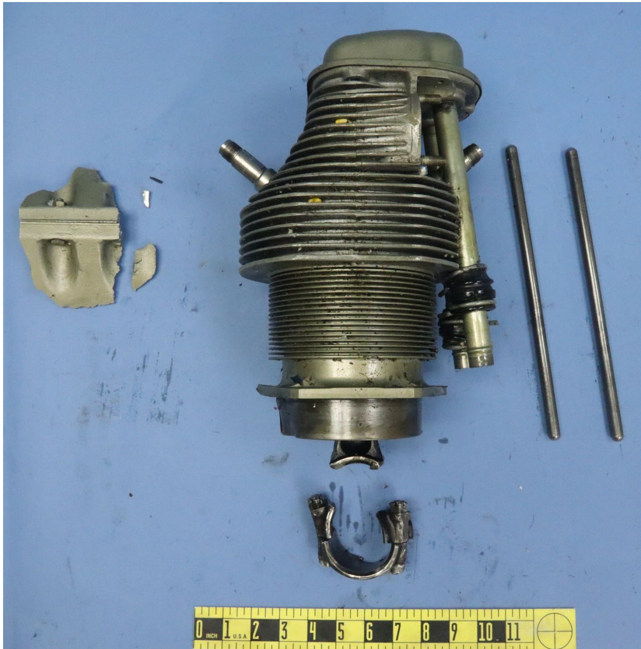
Figure 1. The cylinder, disconnected pushrods, and fractured connecting rod and engine case remnant.
