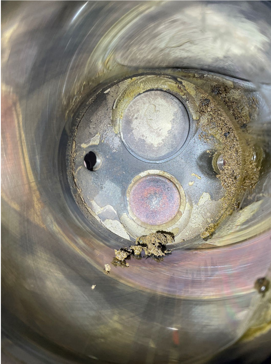
Figure 2. Sand Debris Cylinder number 2
