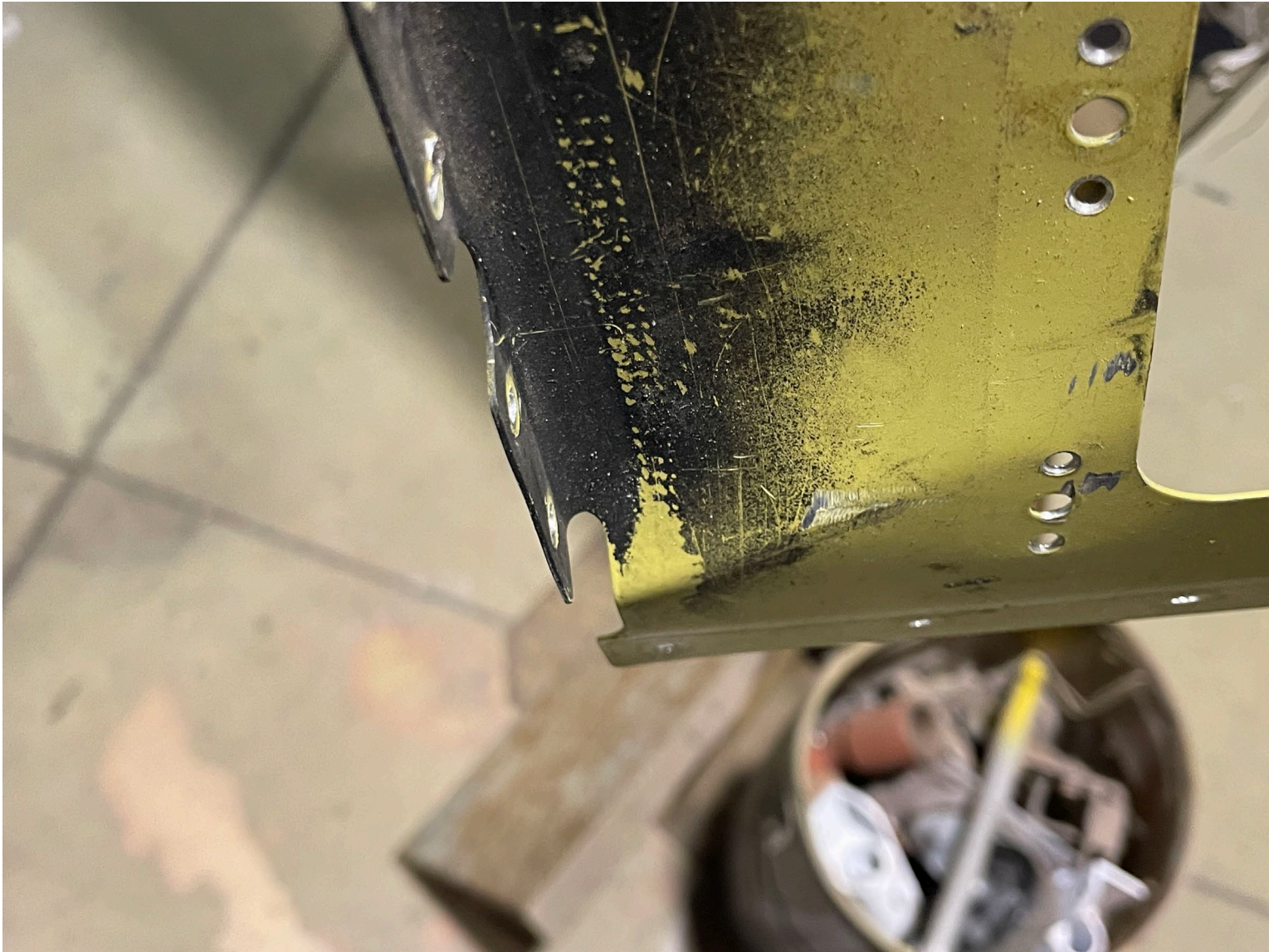
Photograph 1 - Bent Bulkhead (Courtesy of Federal Aviation Administration)
