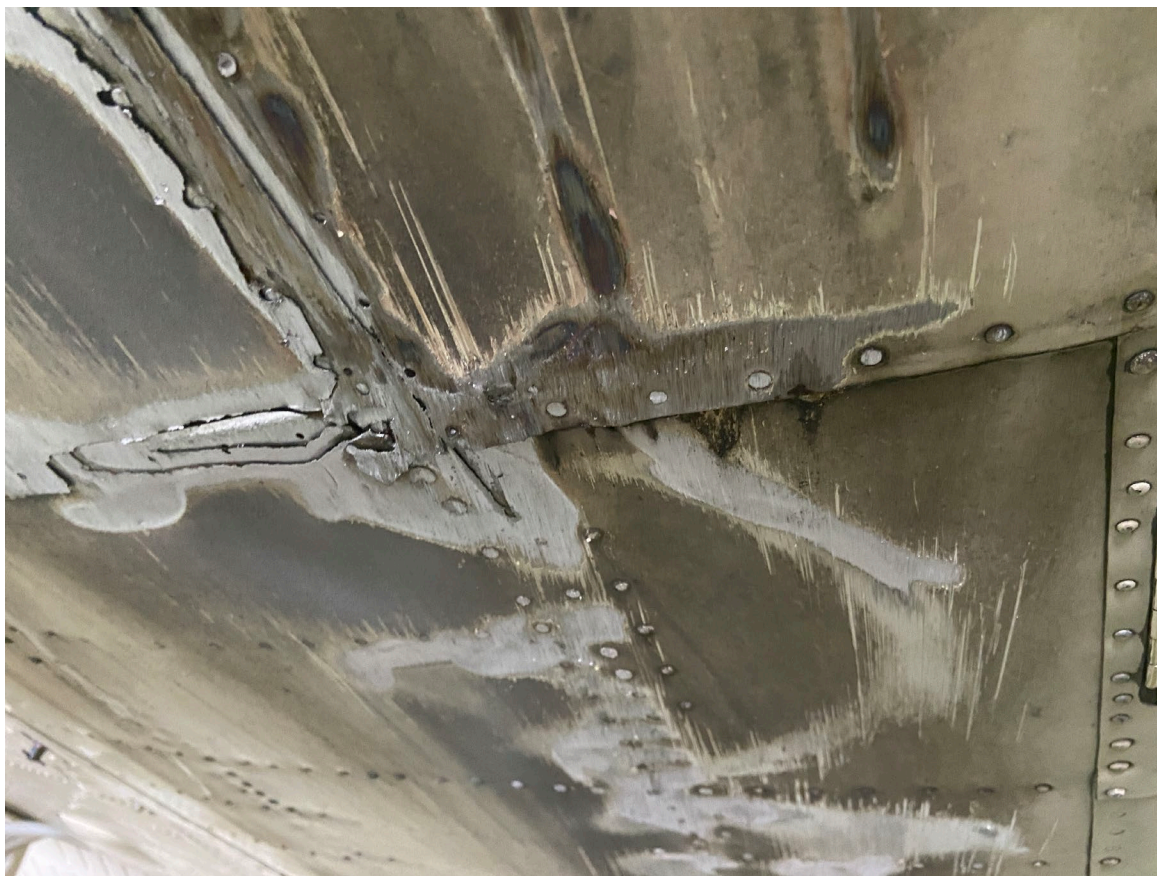
Photograph 2 - Abrasion damage to the lower fuselage (Courtesy of Federal Aviation Administration)
