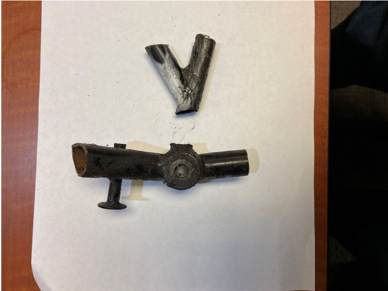
Photograph 3 - View of a portion of the engine mount removed from the airplane (courtesy of the Federal Aviation Administration)
