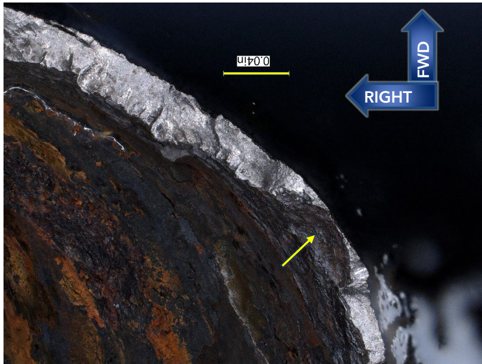
Figure 5. Area (indicated with an unlabeled arrow) where wall loss from corrosion extended nearly through the thickness.
