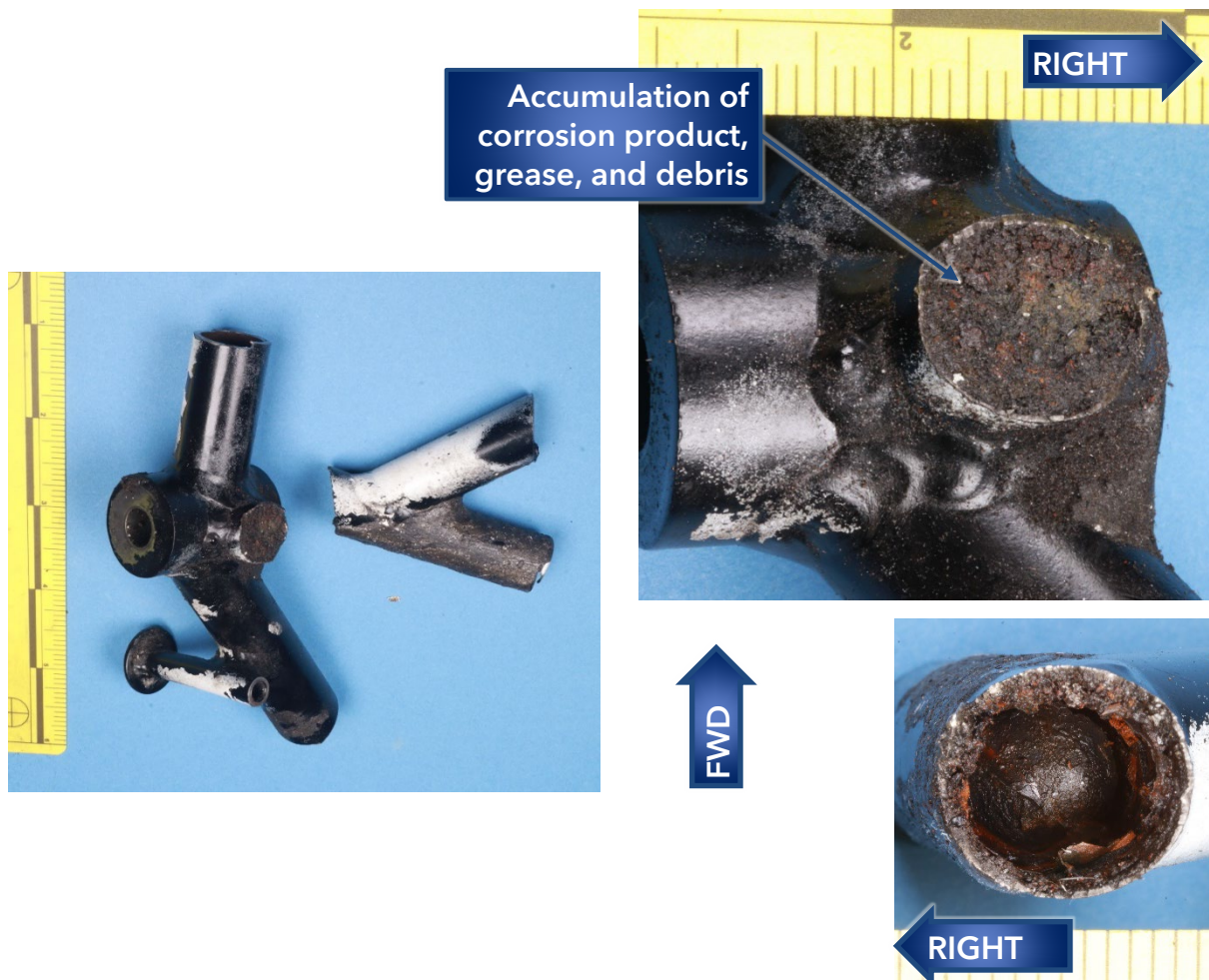
Figure 2. Closer views of the fracture surfaces as received.
