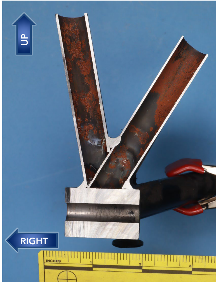
Figure 9. Aft side of the left foot and vertical tube members after cutting to expose the interior surfaces of the vertical tubes.
