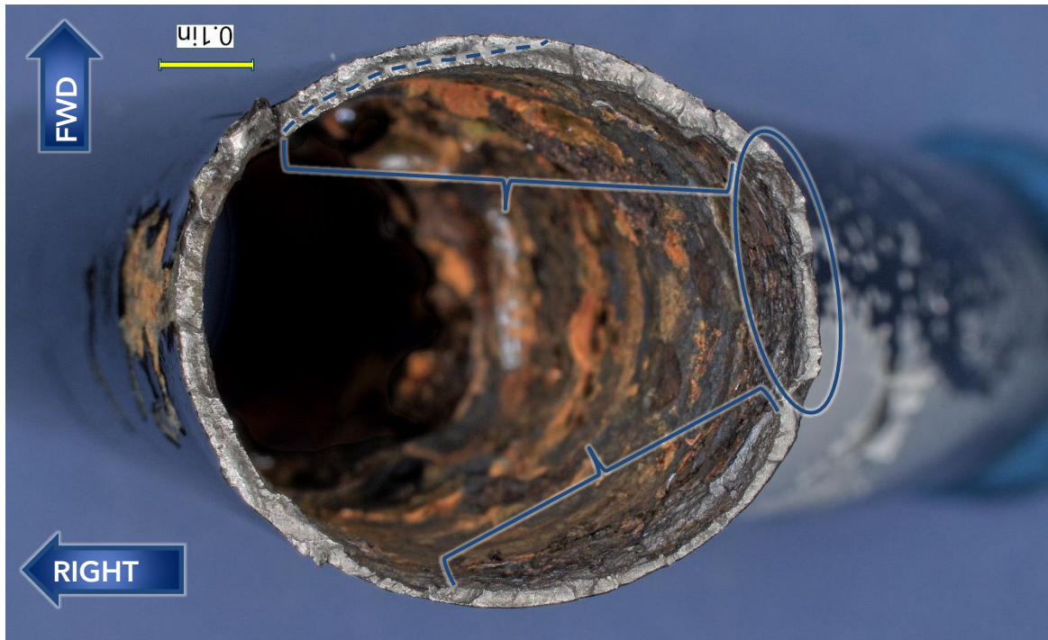
Figure 3. Upper fracture surface after degreasing and ultrasonic cleaning. Brackets indicate multiple fatigue origins extending through thickness or to the fatigue boundary indicated with a dashed line. A circle indicates a damaged area with obliterated fracture features on the left side of the fracture.
