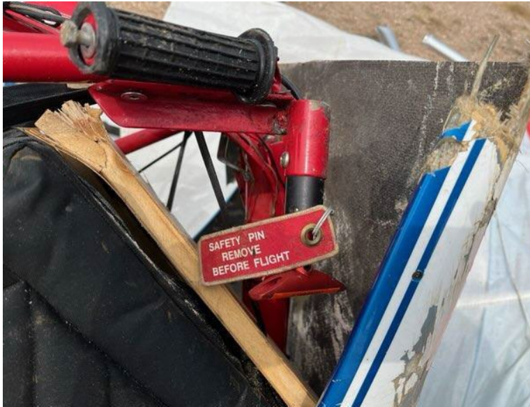
Figure 8. Ballistic Recovery System Safety Pin (Provided by FAA)
