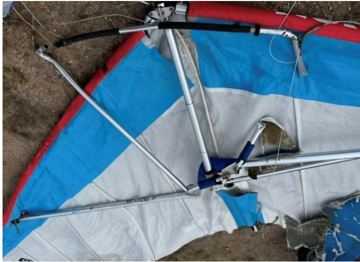
Figure 2. Control Bar and Sail (Provided by FAA)
