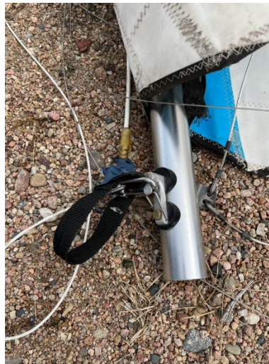
Figure 5. Back End of Keel (Provided by FAA)
