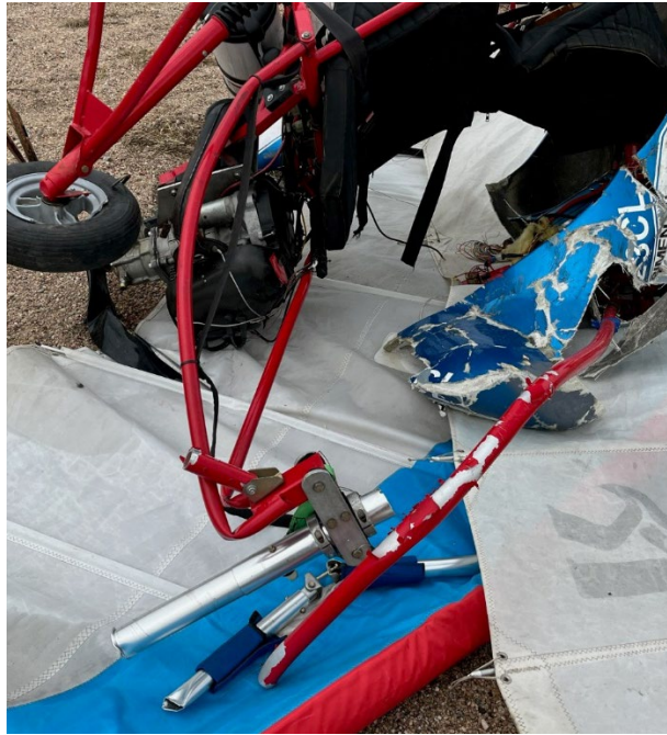
Figure 4. Hang Point and Mast (Provided by FAA)
