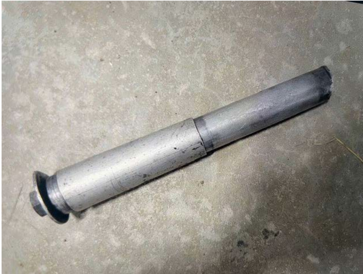
Photograph 4 - Fractured Left Axle (Courtesy of FAA)
