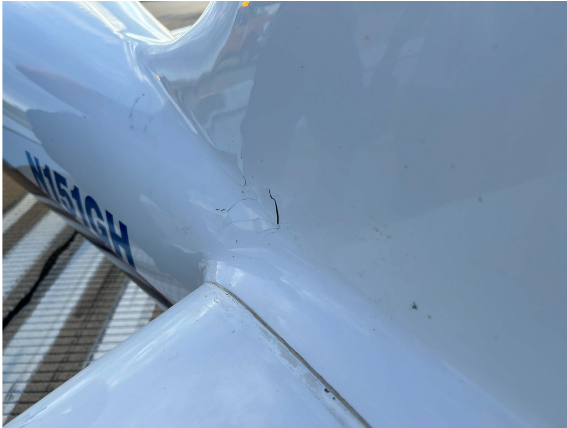
Photograph 2 - Substantial Damage on Fuselage Adjacent to Left Horizontal Stabilizer (Courtesy of FAA)
