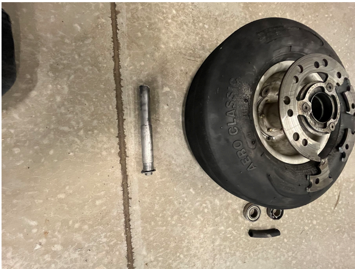
Photograph 3 - Separated Left Wheel Assembly (Courtesy of FAA)
