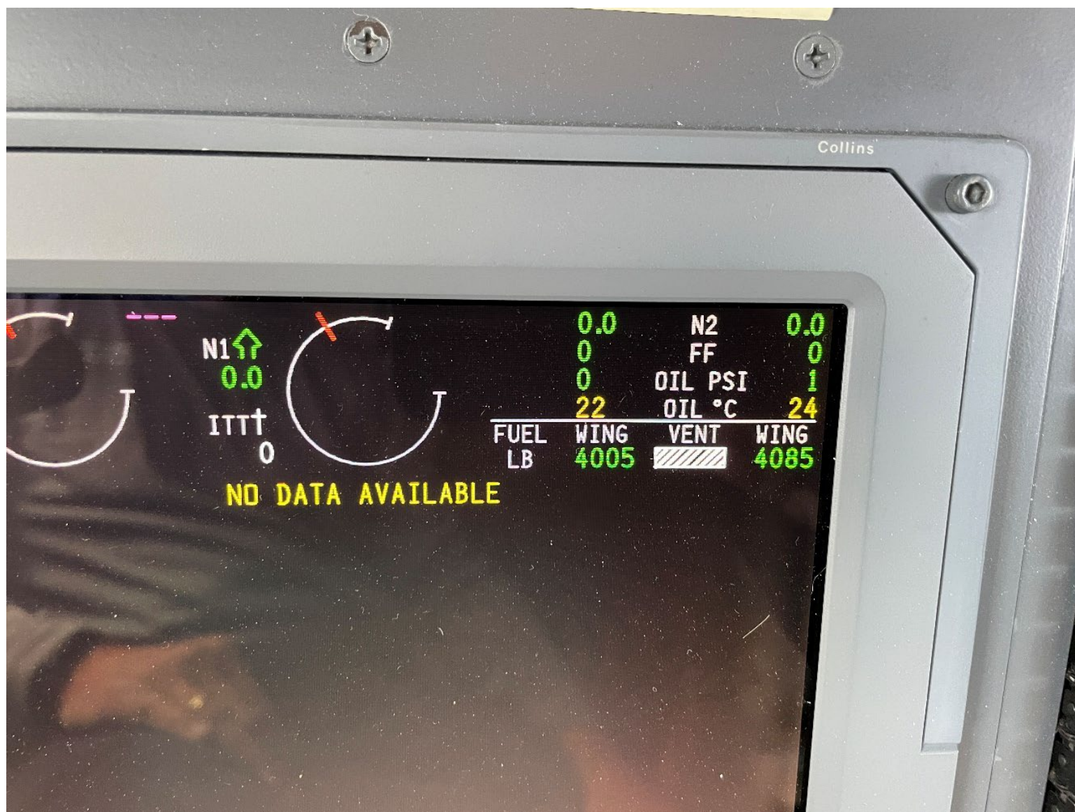
Photograph 14 - View of an electronic cockpit display showing the fuel onboard after the accident
