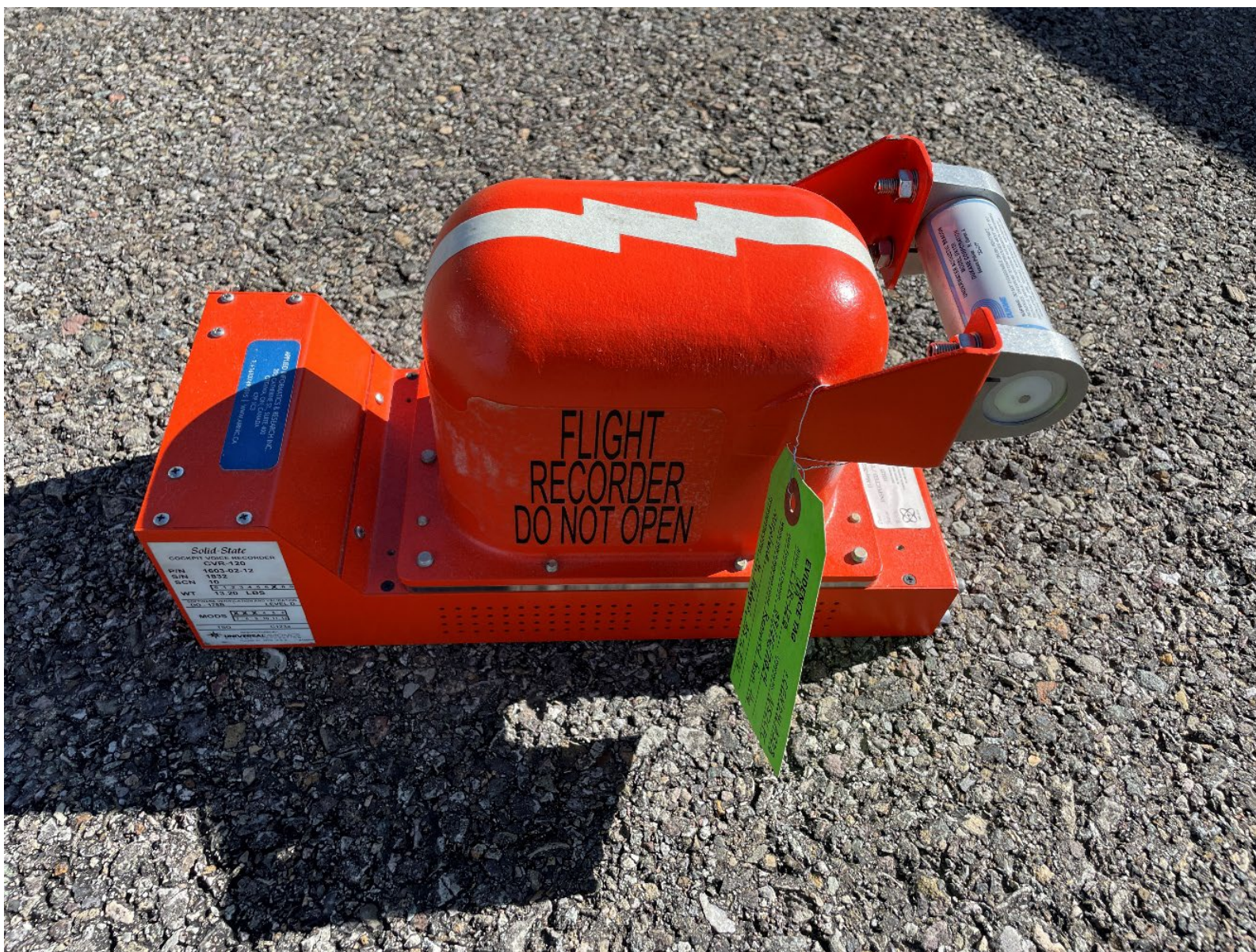
Photograph 15 - View of the cockpit voice recorder removed from the airframe
