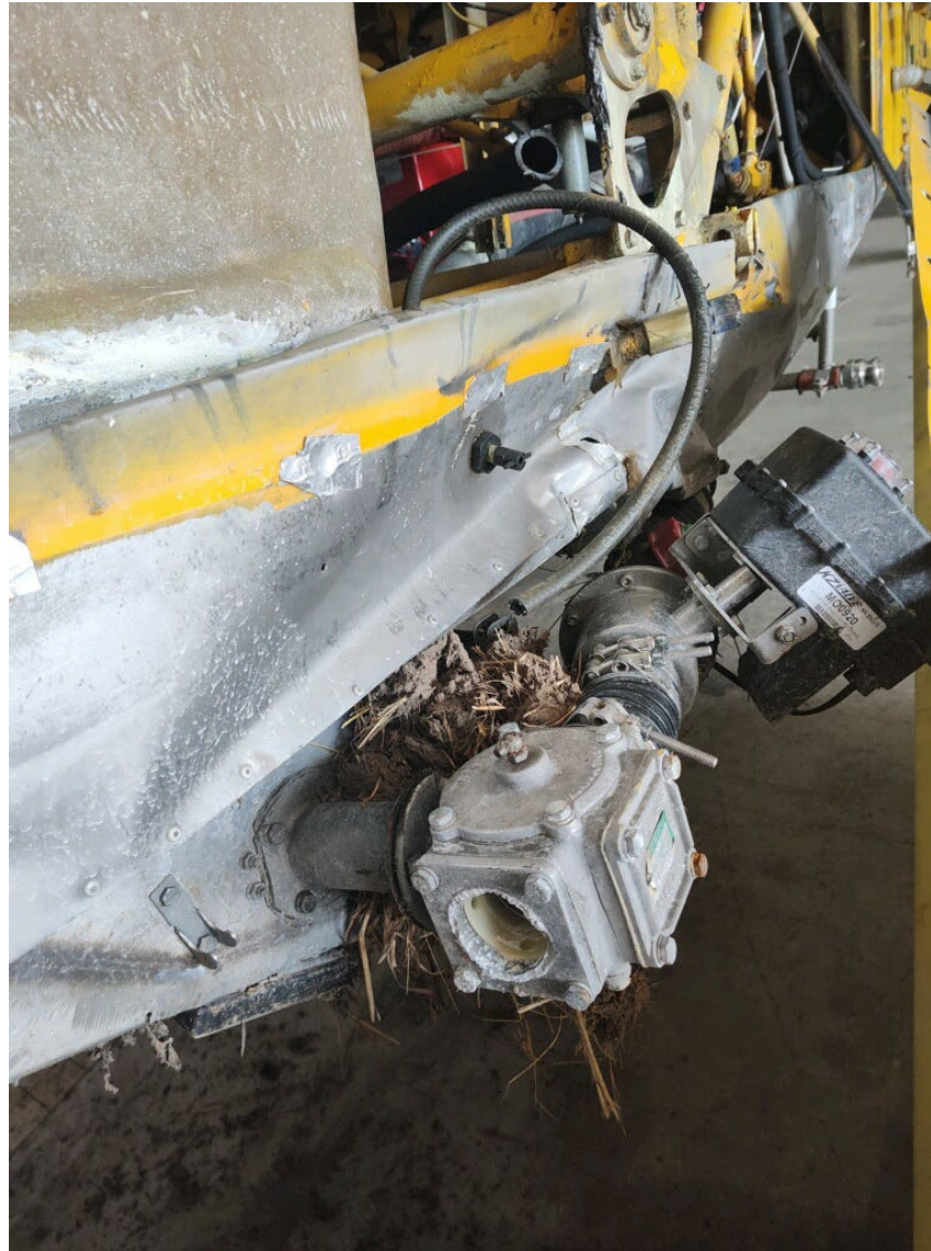
Photograph 6 - View of the substantial damage sustained to the left side of the lower fuselage (courtesy of the operator)
