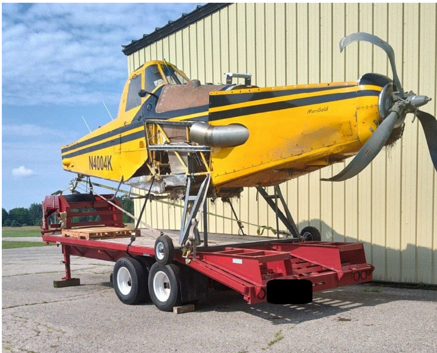
Photograph 9 - View of the fuselage with both wings, the landing gear, and the empennage removed (courtesy of the operator)
