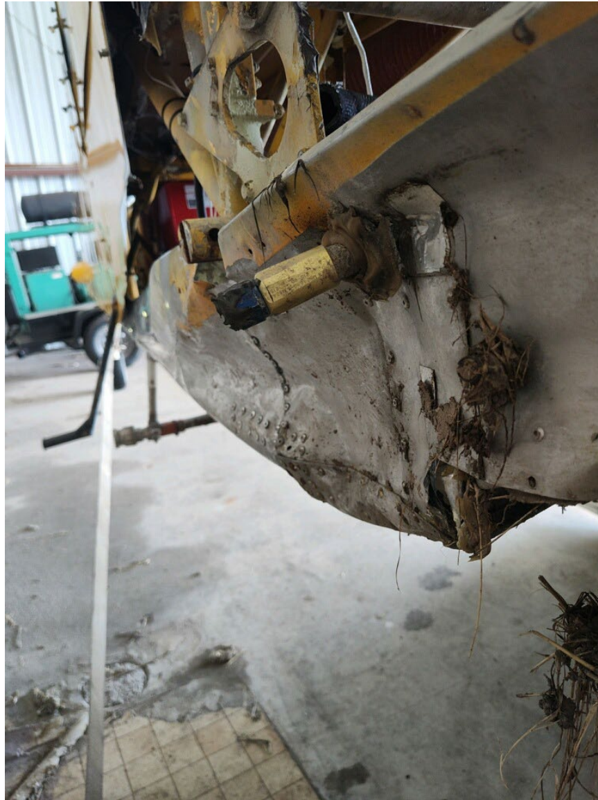
Photograph 5 - View of the substantial damage sustained to the right side of the lower fuselage (courtesy of the operator)
