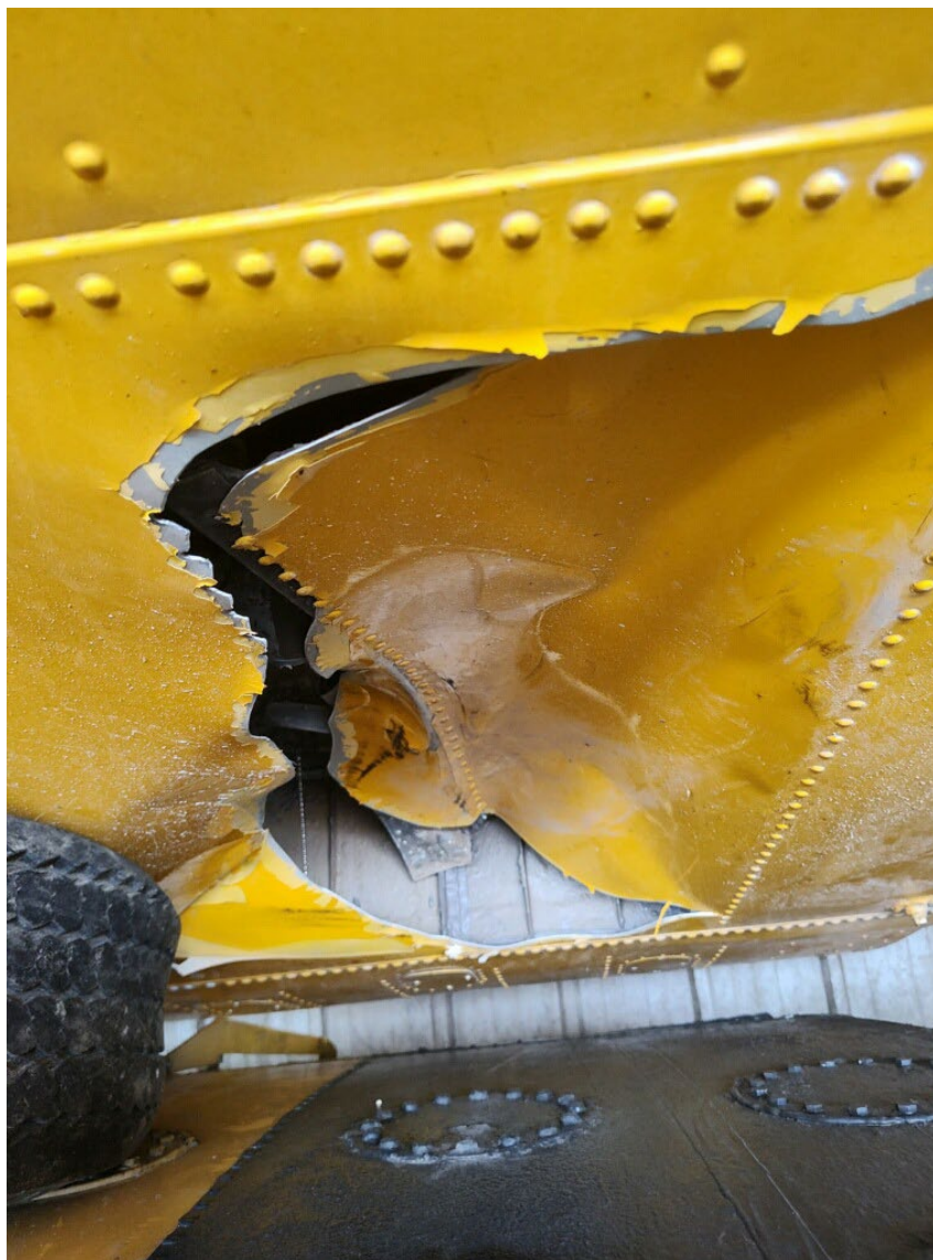
Photograph 7 - View of the substantial damage sustained to the underside of the right wing (courtesy of the operator)
