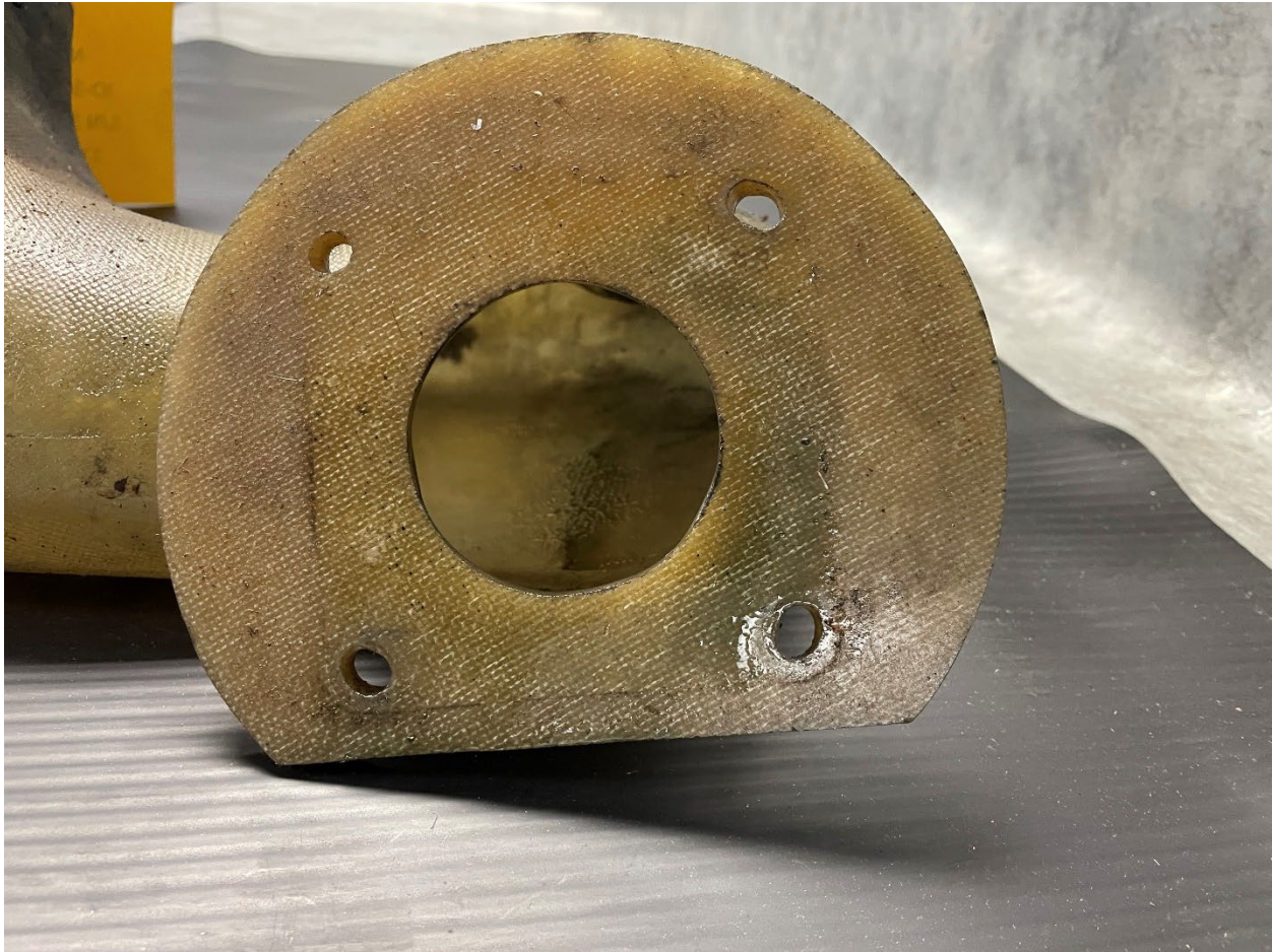
Figure 1. Fiberglass snorkel mount holes to throttle body assembly.
