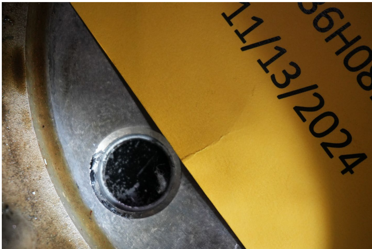
Figure 9. Damage from crankshaft bushing on the rear of the starter ring support.
