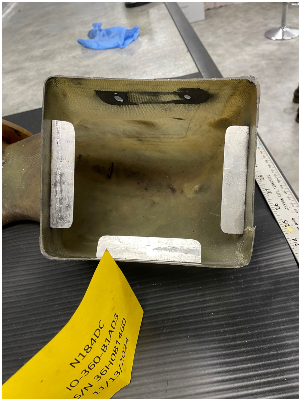
Figure 2. Air filter retaining brackets (rear missing).
