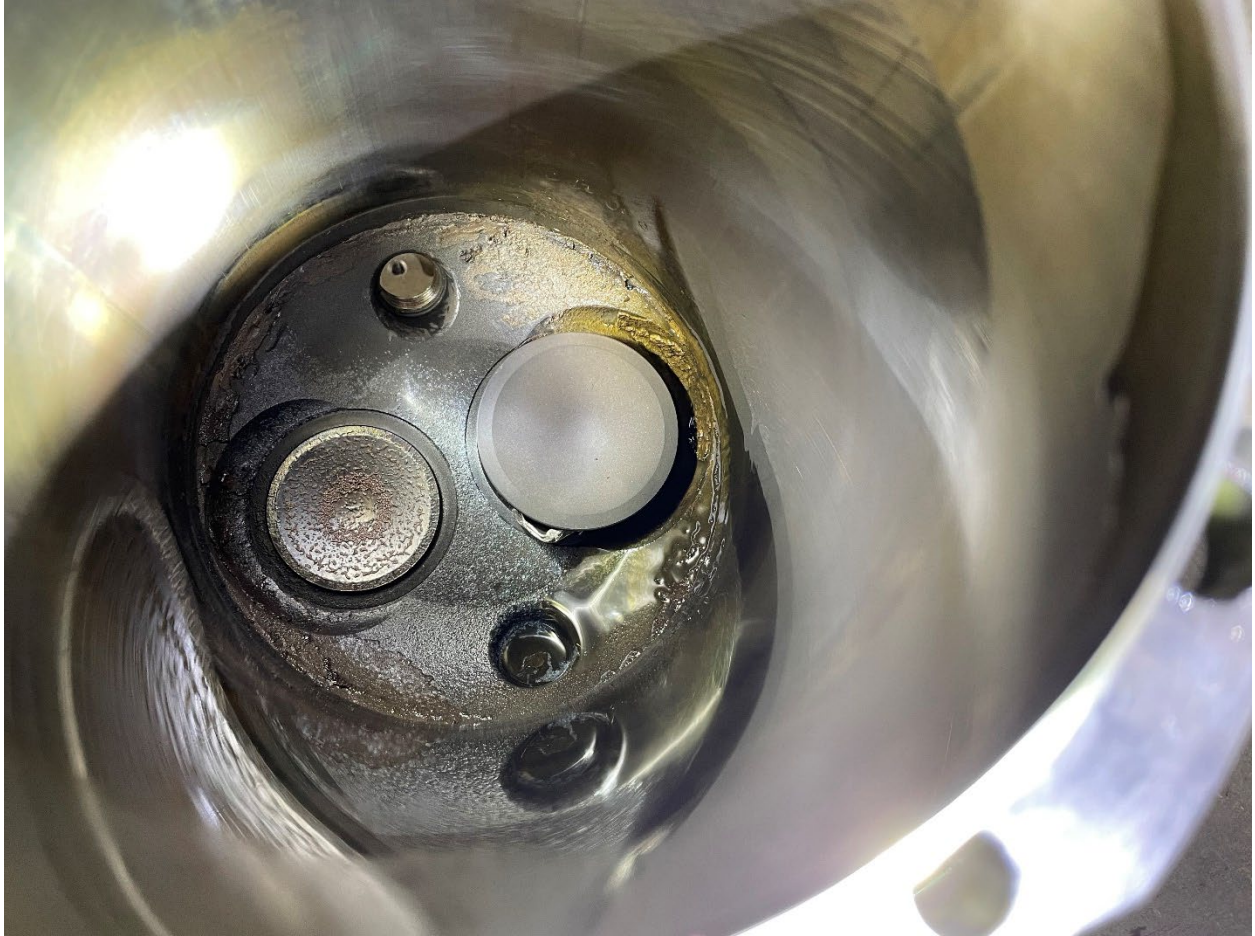
Figure 6. Separated air box bracket found jammed under intake valve seat.
