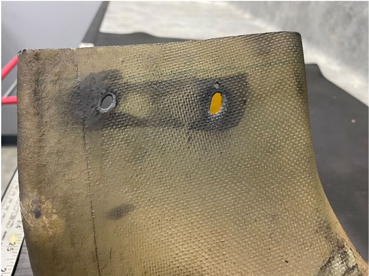
Figure 3. Missing air filter retaining bracket and elongation of attachment rivet holes.
