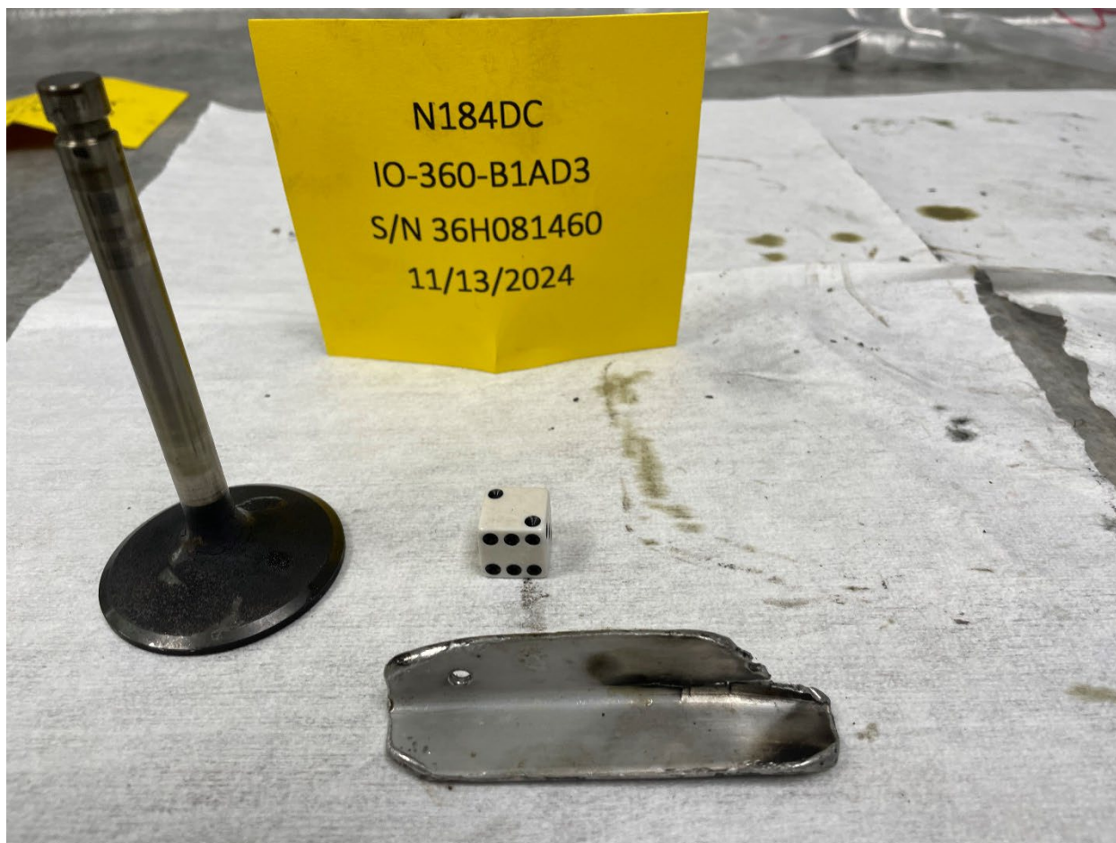
Figure 7. Missing air filter retaining bracket located in No. 2 cylinder.
