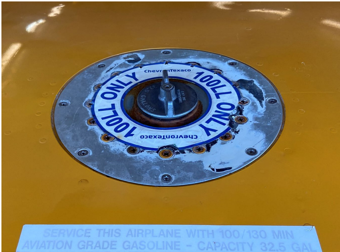
Figure 2. Left Fuel cap installed (note corrosion at the sealing surface).
