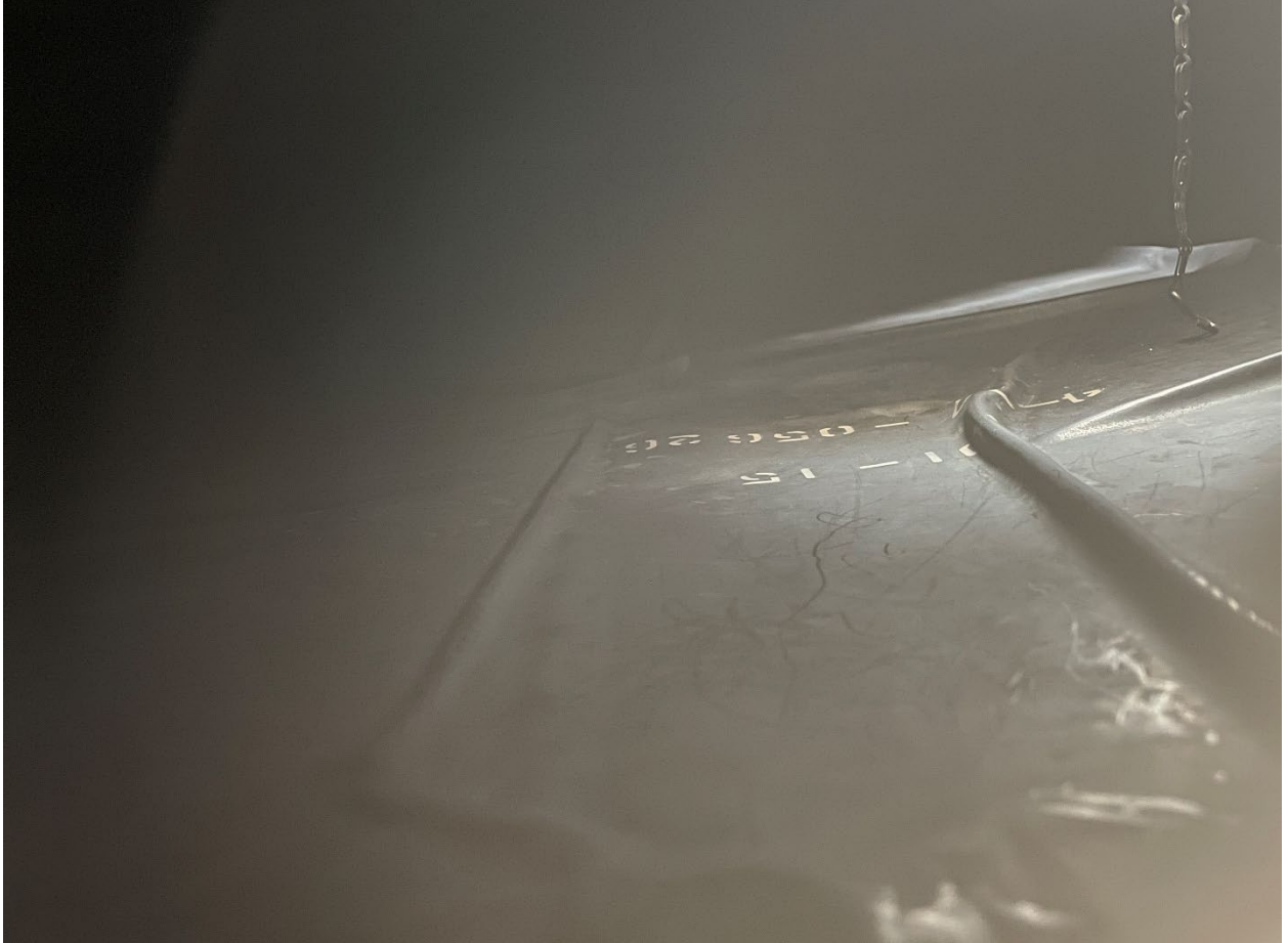
Figure 4. Left wing fuel bladder with wrinkling.
