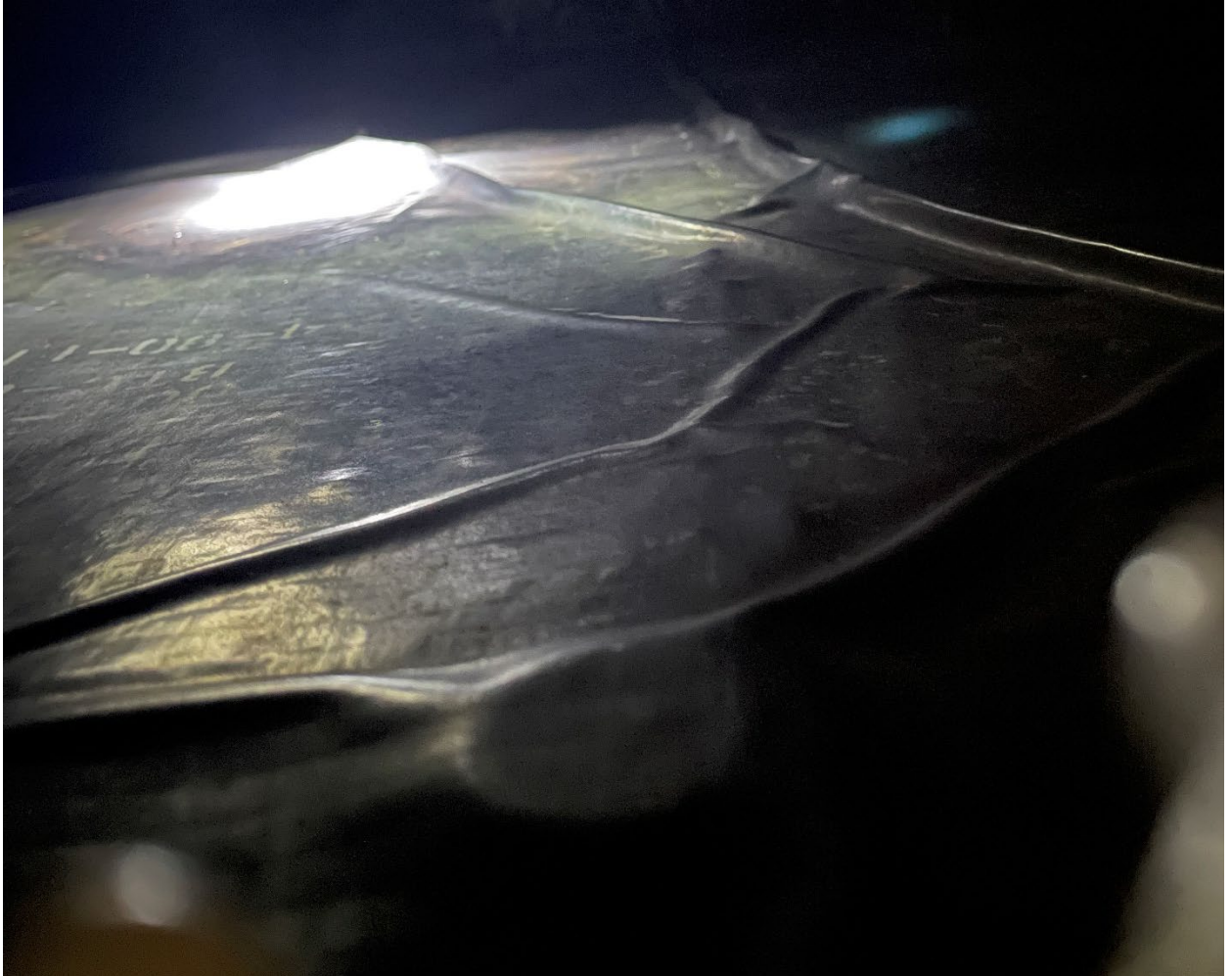
Figure 3. Right wing fuel bladder with wrinkling.
