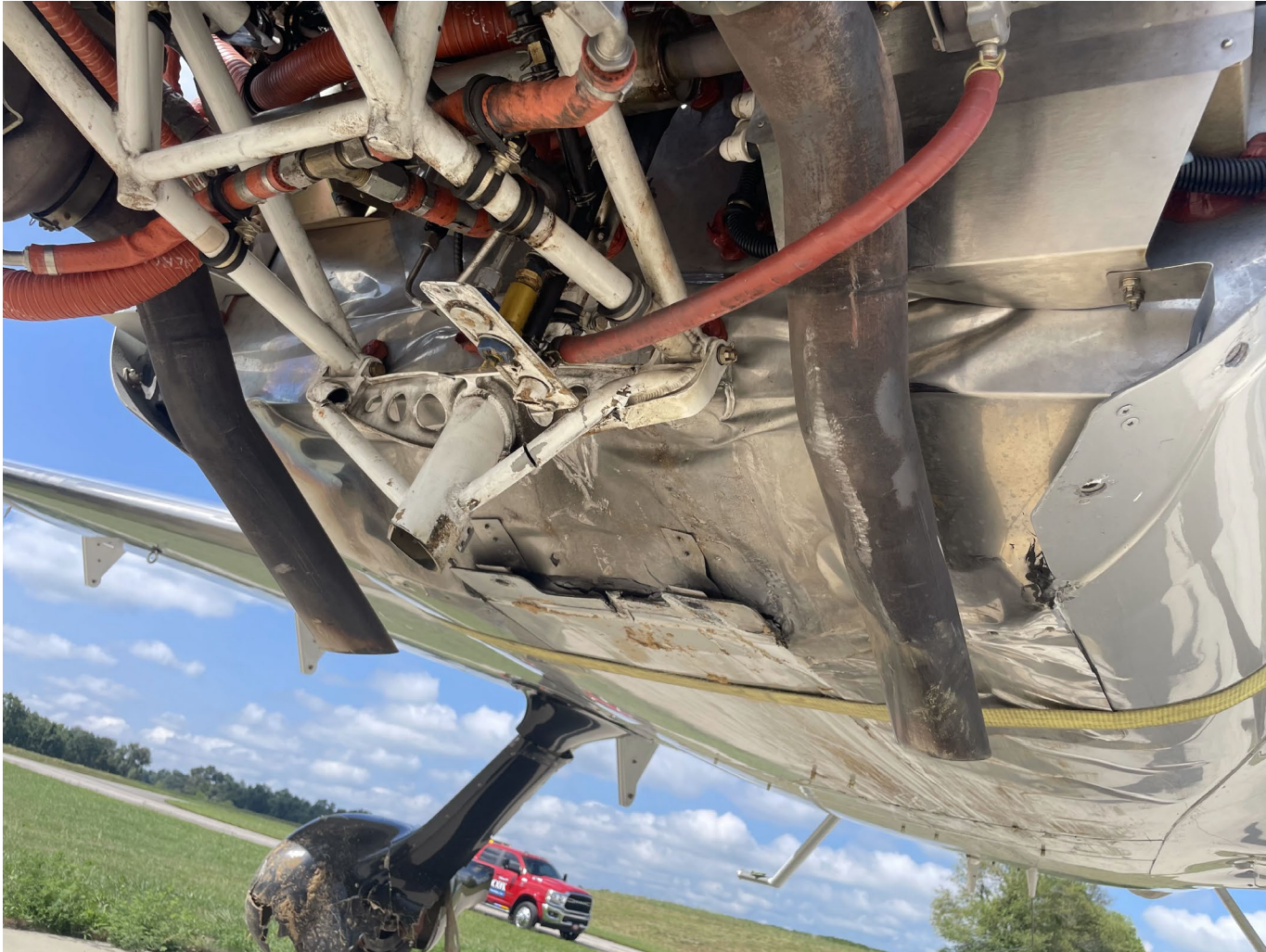
Photograph 1 -Substantial Damage to Firewall and Belly (Courtesy of Lone Mountain Aircraft)
