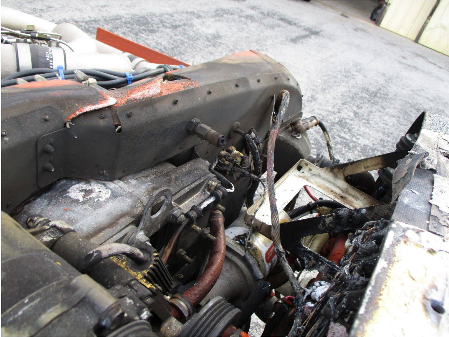
Photograph 4: Engine Compartment Thermal Damage (Courtesy of the Federal Aviation Administration)
