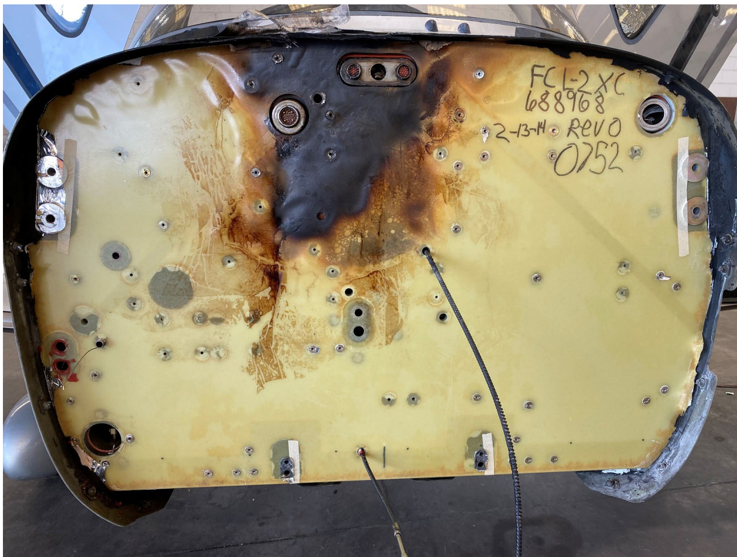
Photograph 6: Firewall Damage (Courtesy of the Federal Aviation Administration)
