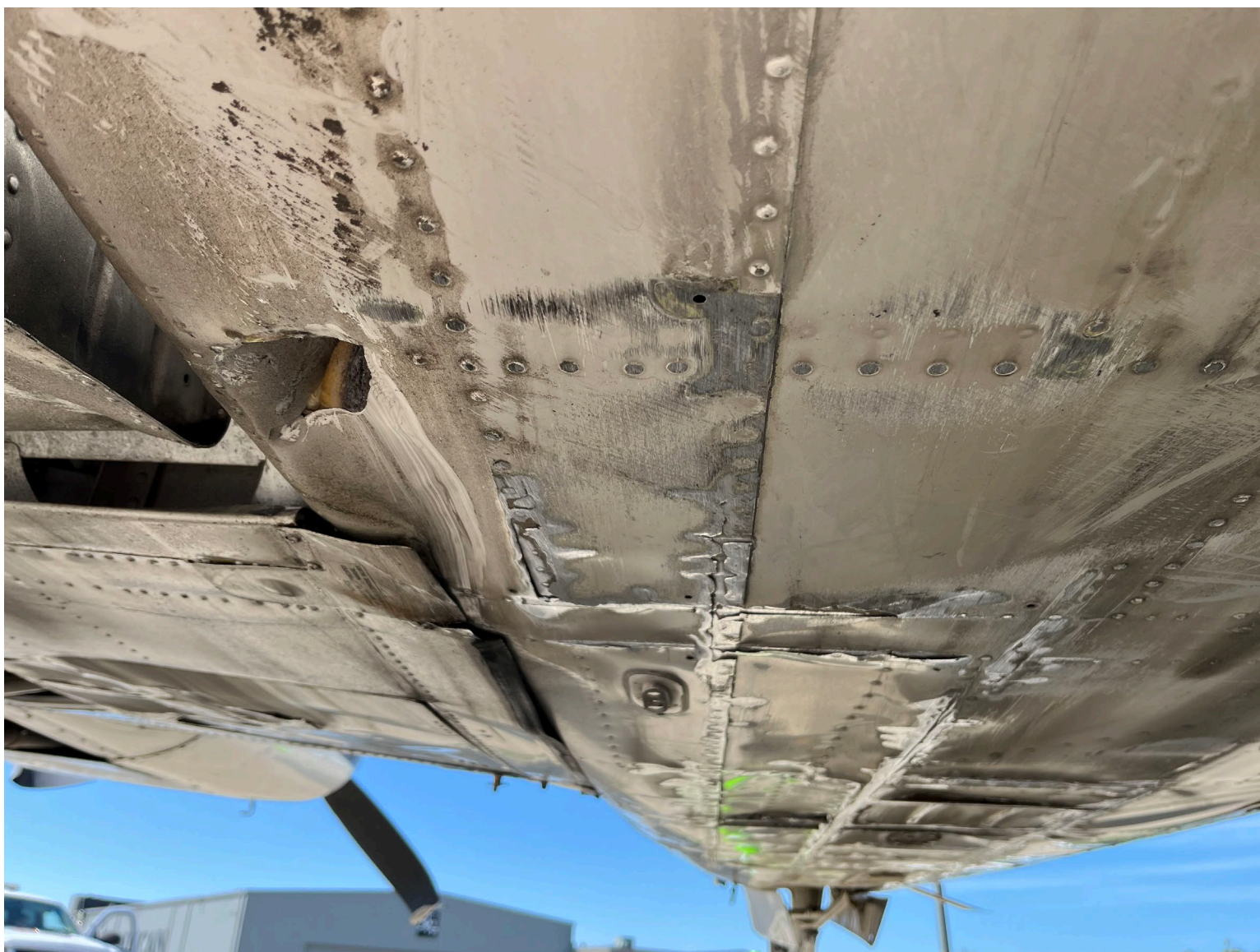
Photograph 2 - Lower Fuselage and Wing Damage (Courtesy of Federal Aviation Administration)
