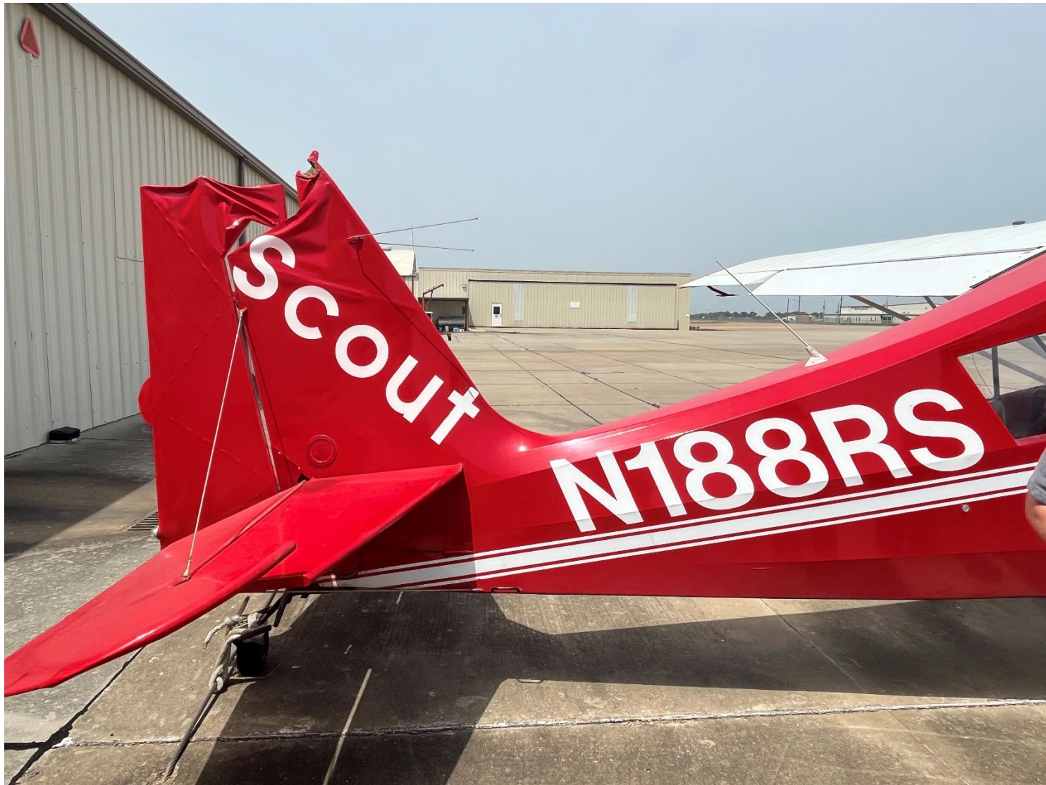
Photograph 2 - Vertical Stabilizer and Rudder Damage (Source - Federal Aviation Administration)
