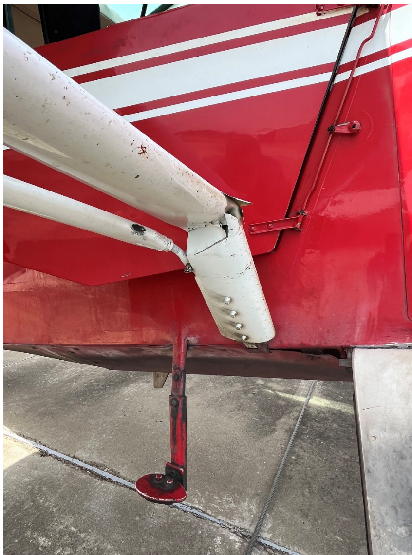
Photograph 1 - Right Wing Strut Damage (Source - Federal Aviation Administration)
