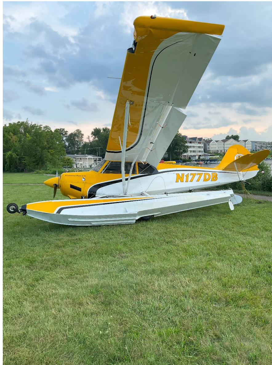
Photograph 2 - Left Wing Strut Substantial Damage (Courtesy of FAA)
