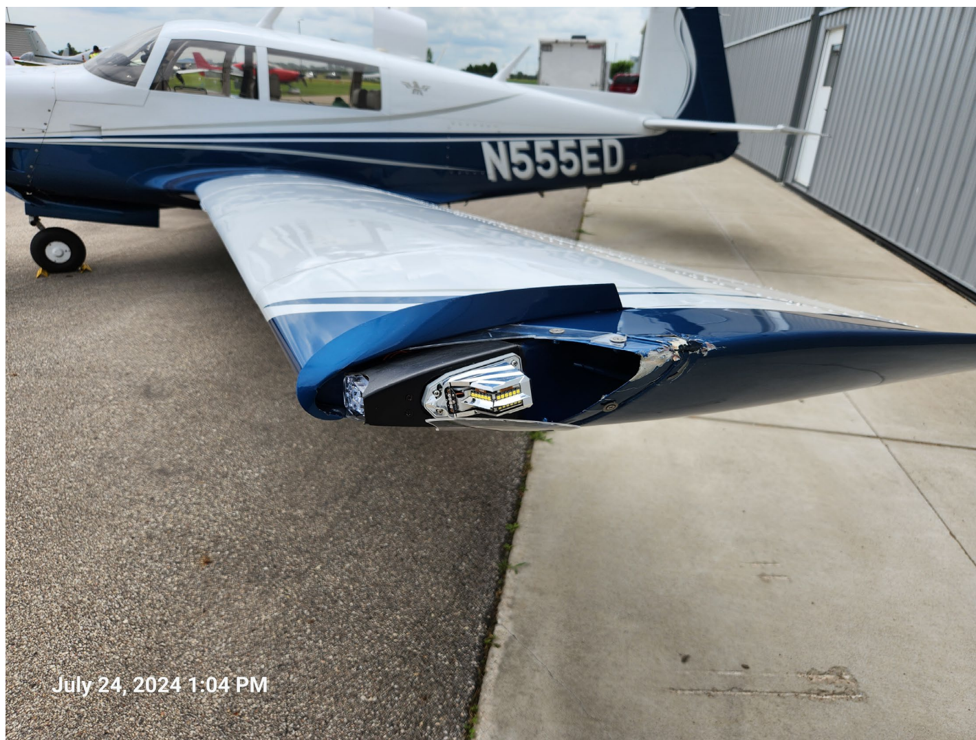
Photograph 2 - Minor Left Wingtip Damage (Courtesy of FAA)
