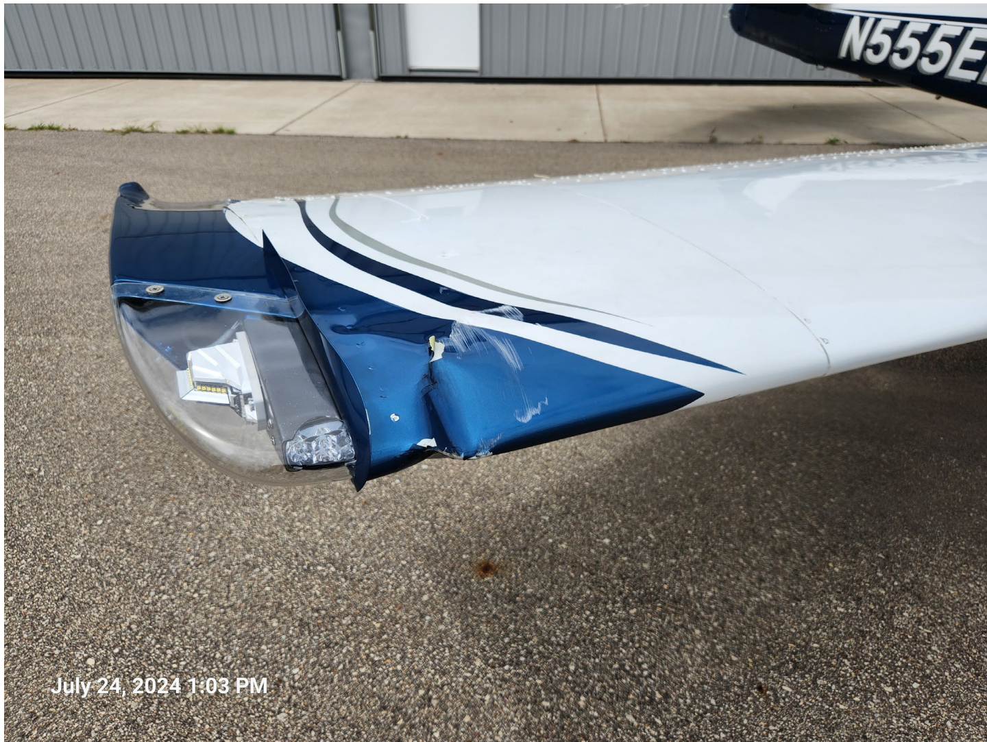
Photograph 1 - Minor Right Wingtip Damage (Courtesy of FAA)
