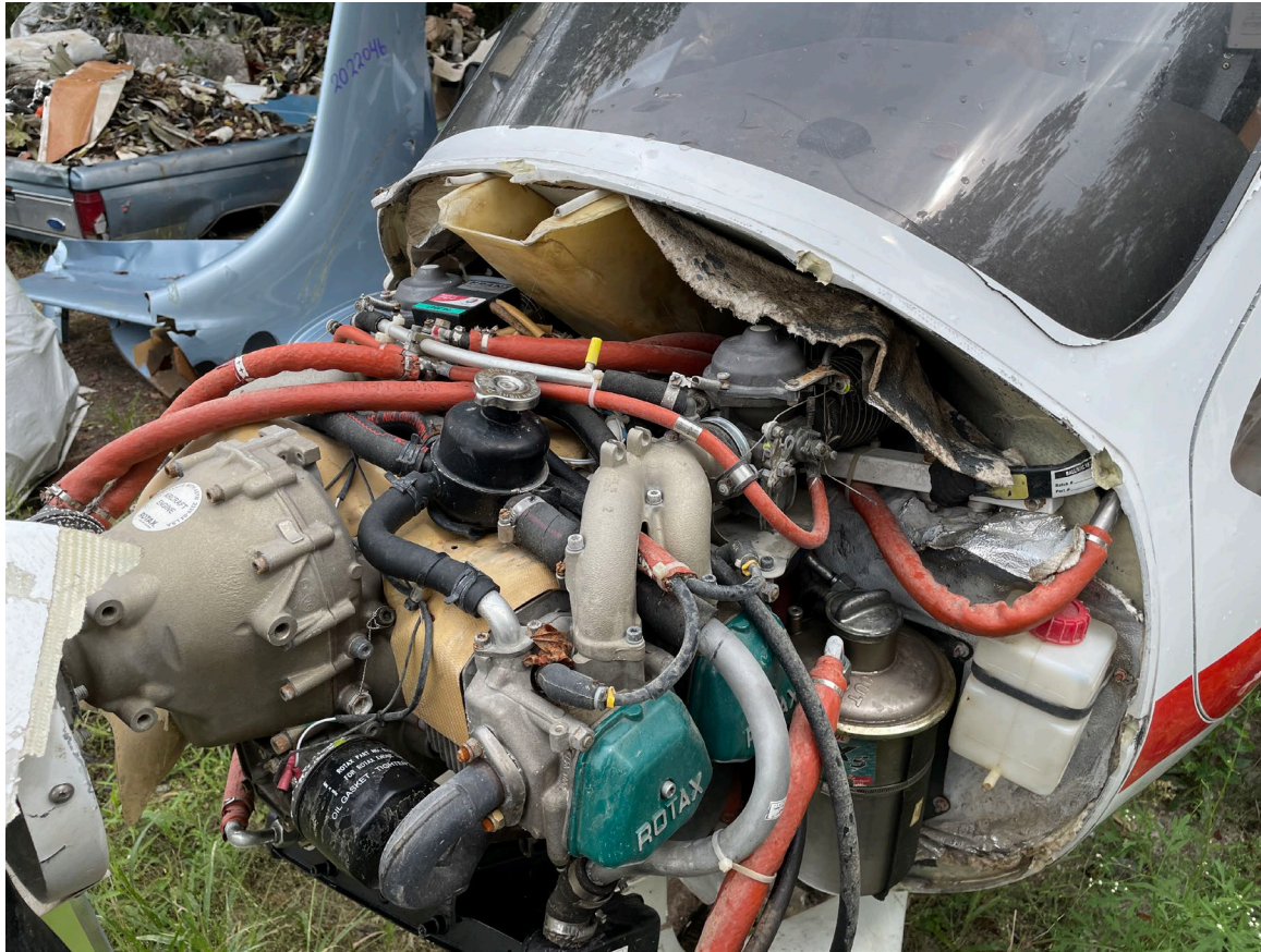
Photograph 2 - Substantial Damage to Firewall (Courtesy of FAA)
