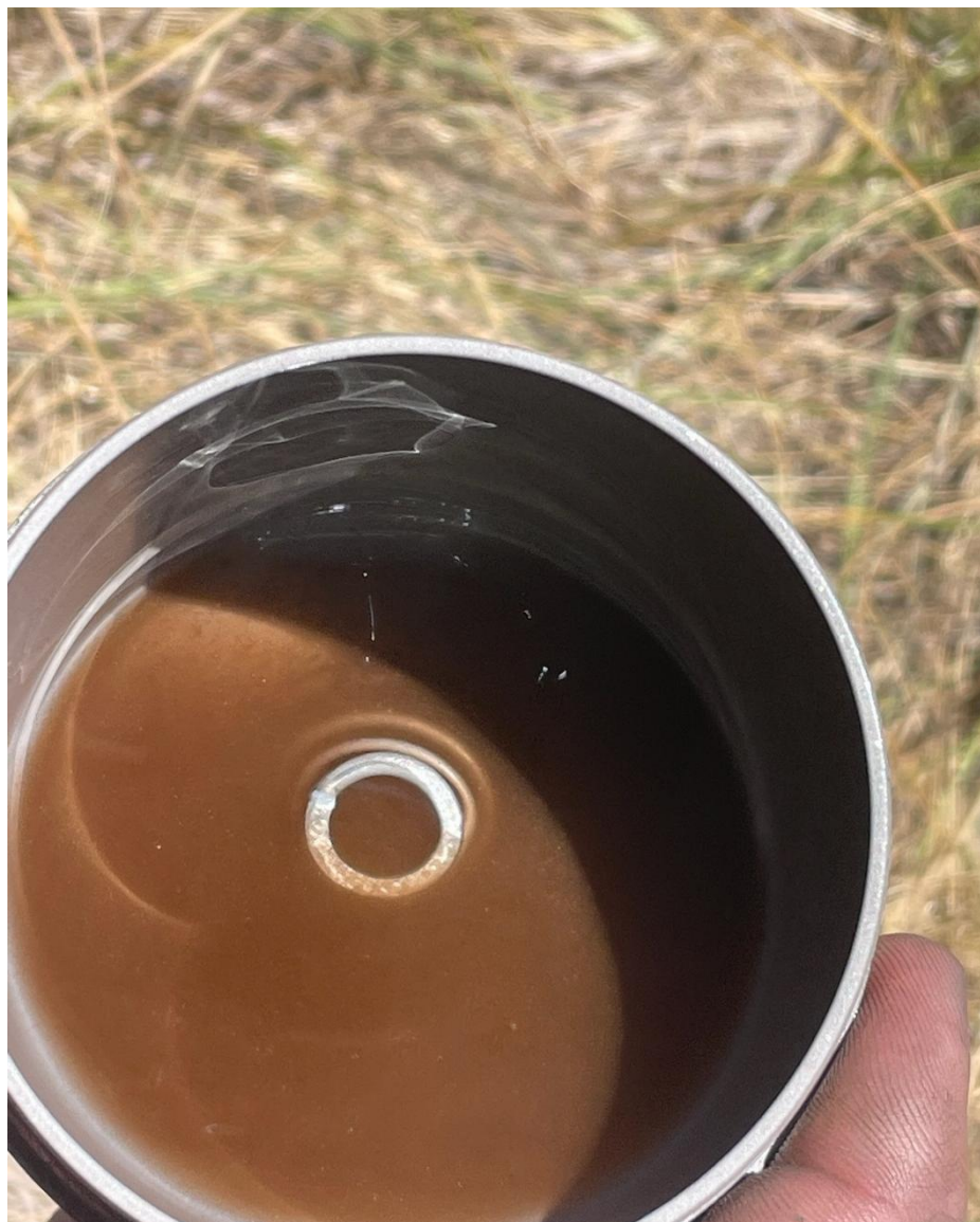
Photograph 3 - Firewall fuel filter bowl (Operator photo)
