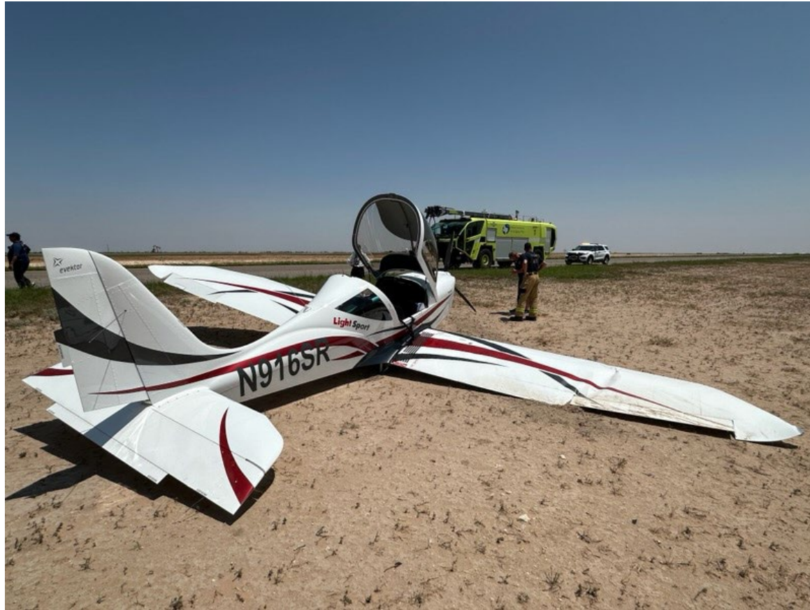
Photograph 2 - Accident airplane with damaged right wing
