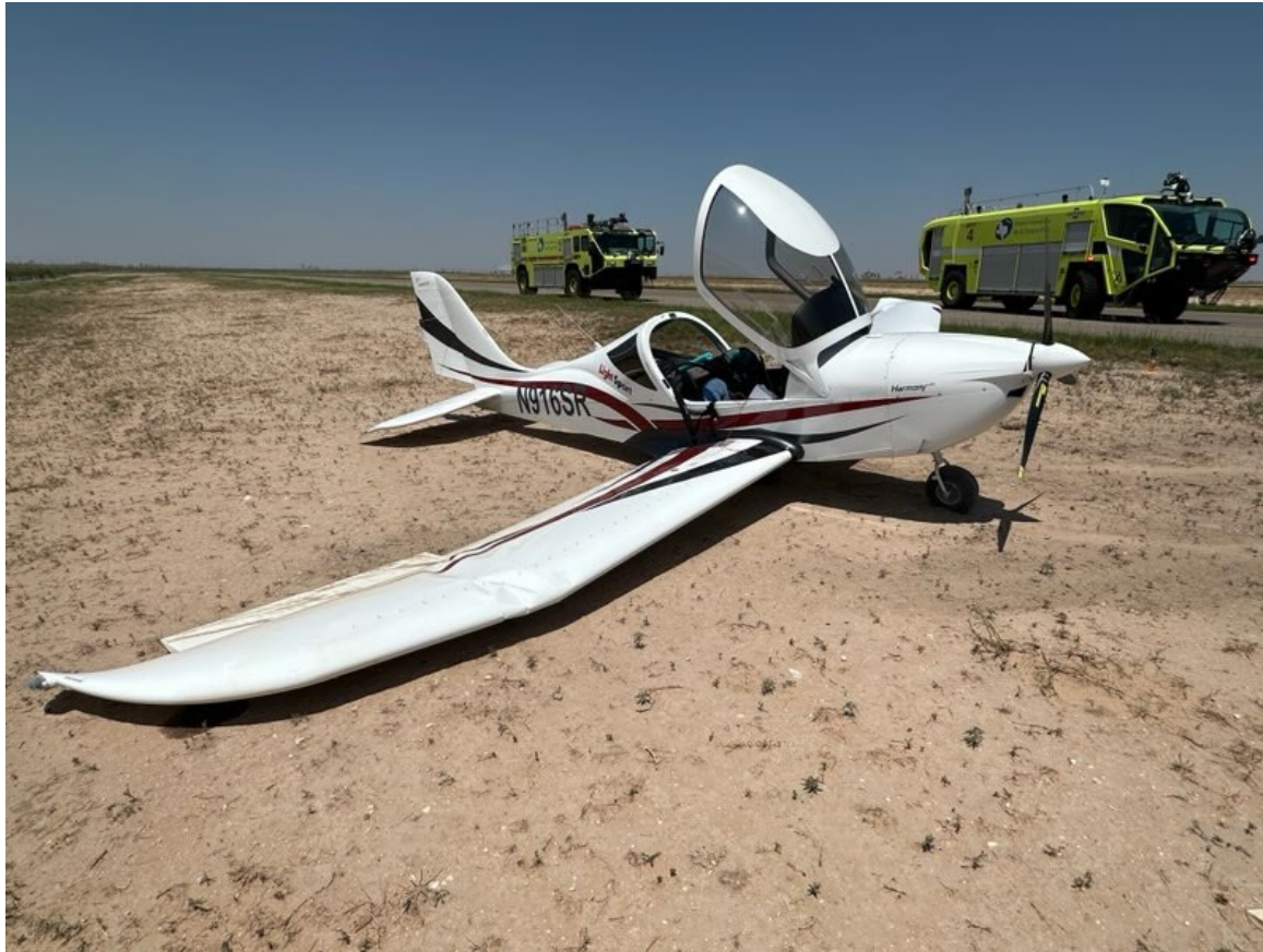
Photograph 1 - Accident airplane with damaged right wing
