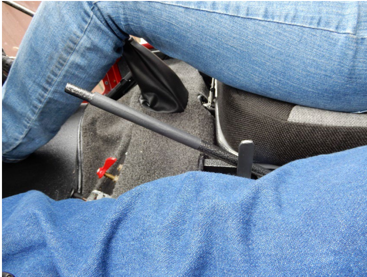
Figure 2. Flap handle on the floor between the right and left seat.
