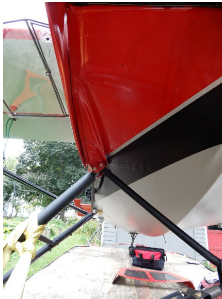
Figure 1. Substantial damage on right side of fuselage
