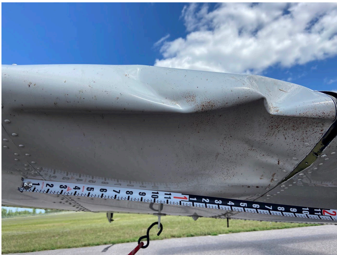
Photograph 2 - Right Wing Substantial Damage (Courtesy of FAA)
